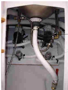
12 V electric bilge pump under basin in aft port head
