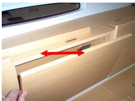
Side lockers opening/ closing system
