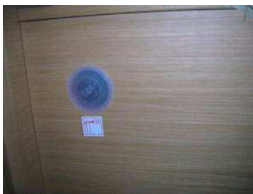
Extinguisher hole located under the companionway step - (Reference 2) A diagram enables it to be found easily
