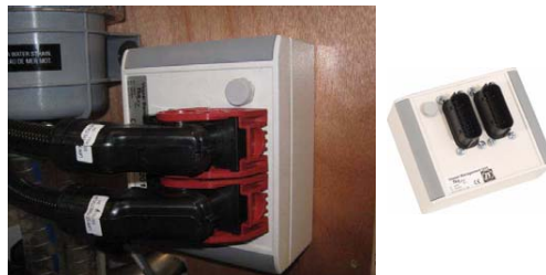
VMU housing (Vessel Management Unit) (Ref 6)
