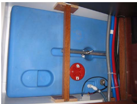
Water tanks - additional Location: Port saloon & Starboard Capacity: 2 x 165 litre
