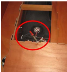
Supply valve Extra tank (Ref 1)
