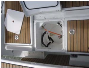
Gas cylinder locker
