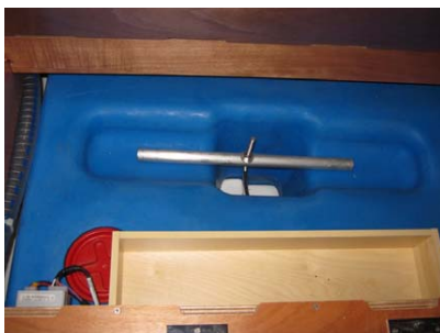
Water tanks - additional Location: Port saloon & Starboard Capacity: 2 x 165 litre
