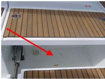
Storage locker for liferaft (not supplied) (Ref 3)
