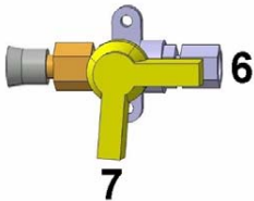
Valve 6 - Open position 7 - Closed position
