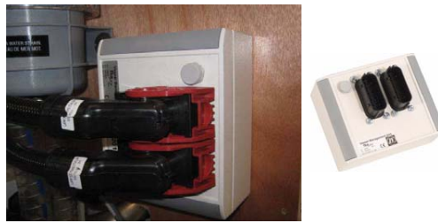
VMU housing (Vessel Management Unit) (Ref 6)
