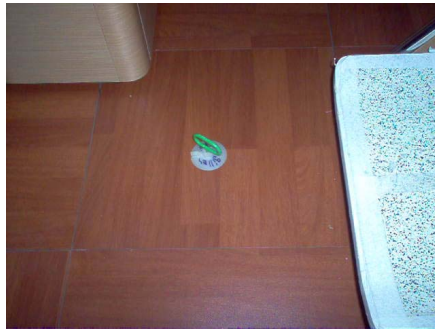
Suction-cup system to lift floors
