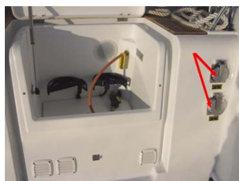
Shore power socket 30A & 63A (Ref 1)
