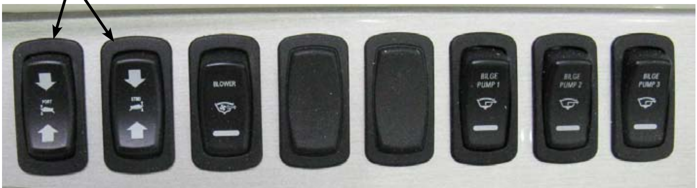
Trim Tab switches
