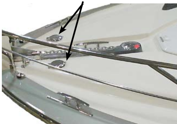
Bow Anchor Switches (lift covers to access)
