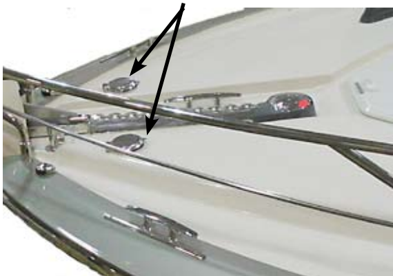
Bow Anchor Switches (lift covers to access)
