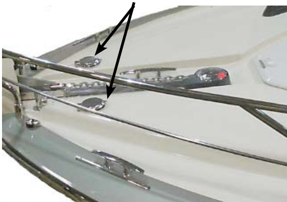
Bow Anchor Switches (lift covers to access)
