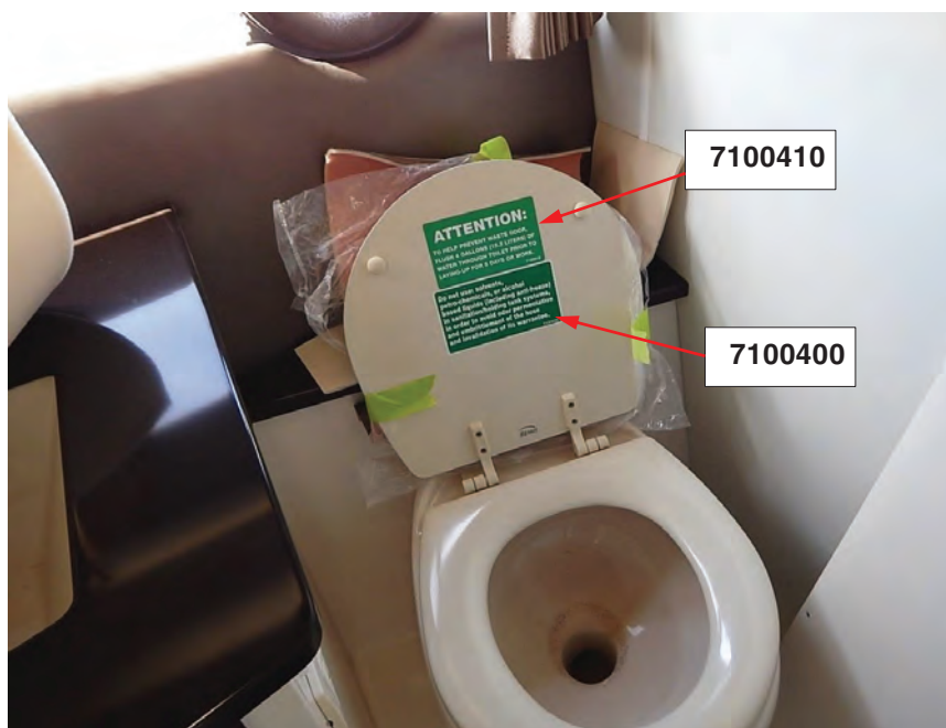
Figure 2-13 – Labels Applied to Underside of Toilet Seat Cover
