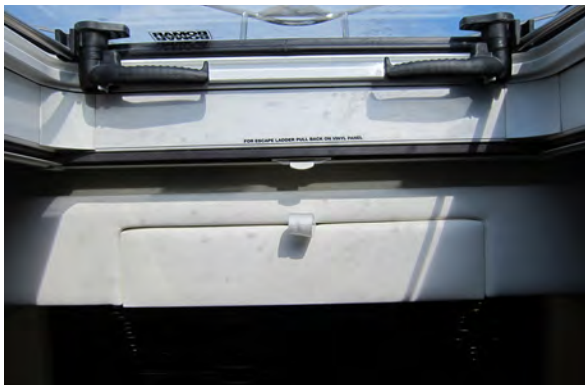
Figure 4-1 – Emergency Ladder Location
