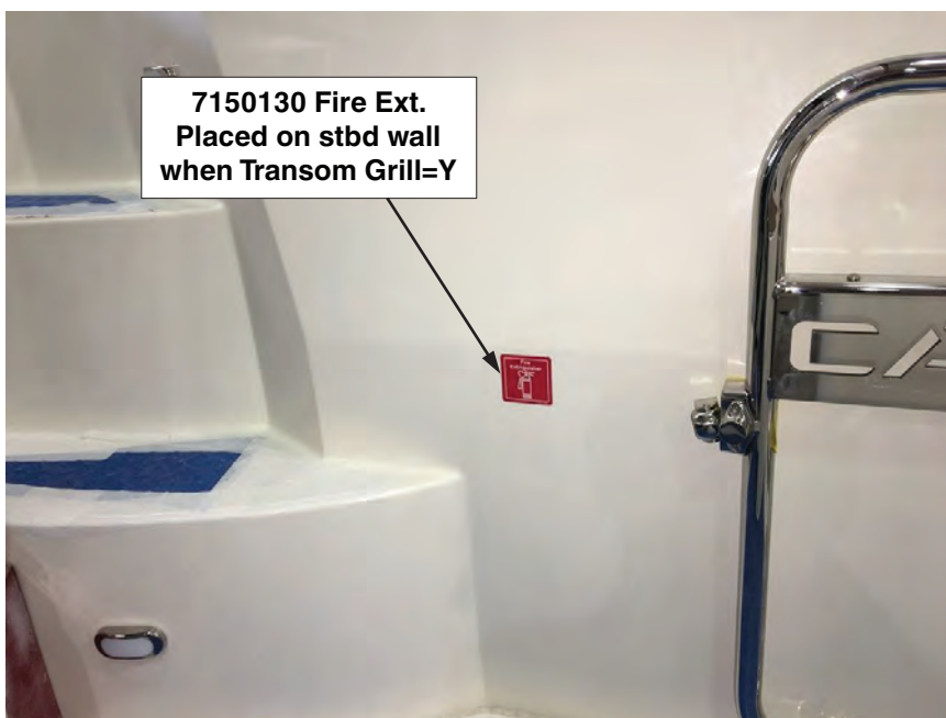
Figure 2-5 – Fire Extinguisher Lable Placed in Cockpit When Transom Grill=Y
