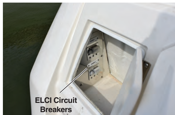
Figure 7-9 – Shore Power Circuit Breakers
