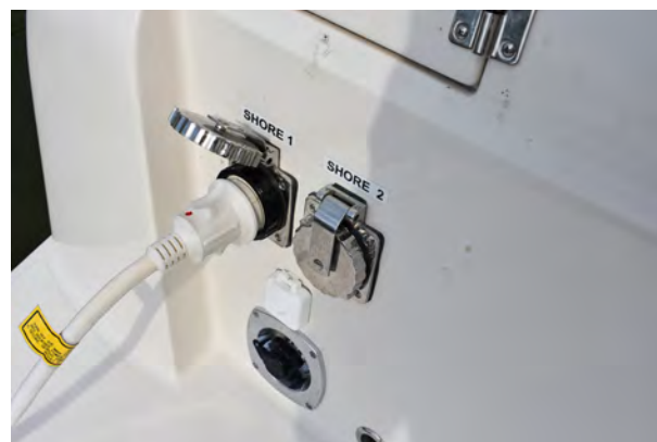
Figure 7-8 – Shore Power Receptacles
