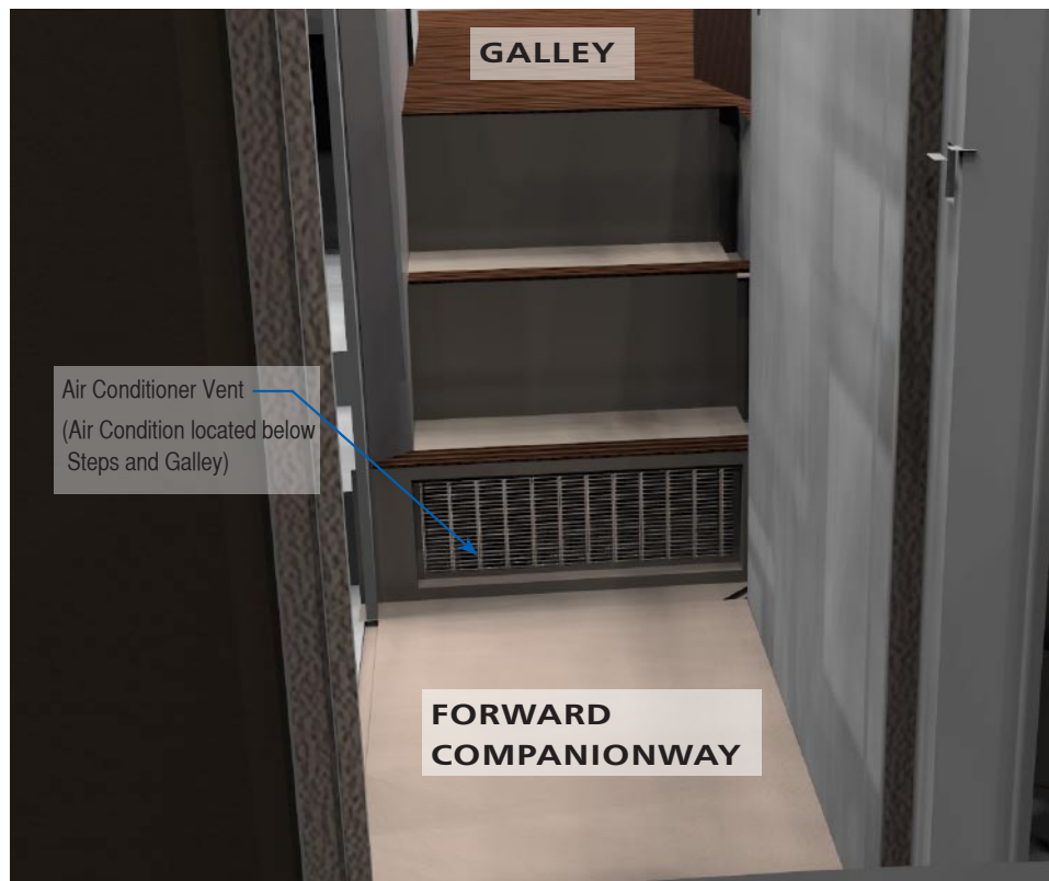
AIR CONDITIONER RETURN VENT
