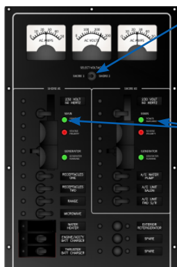
AC CONTROL PANEL
