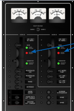
AC CONTROL PANEL
