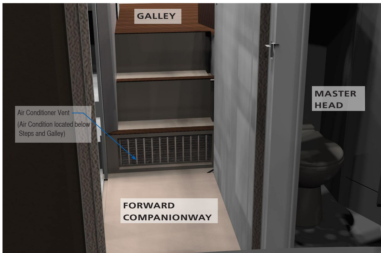
AIR CONDITIONER RETURN VENT
