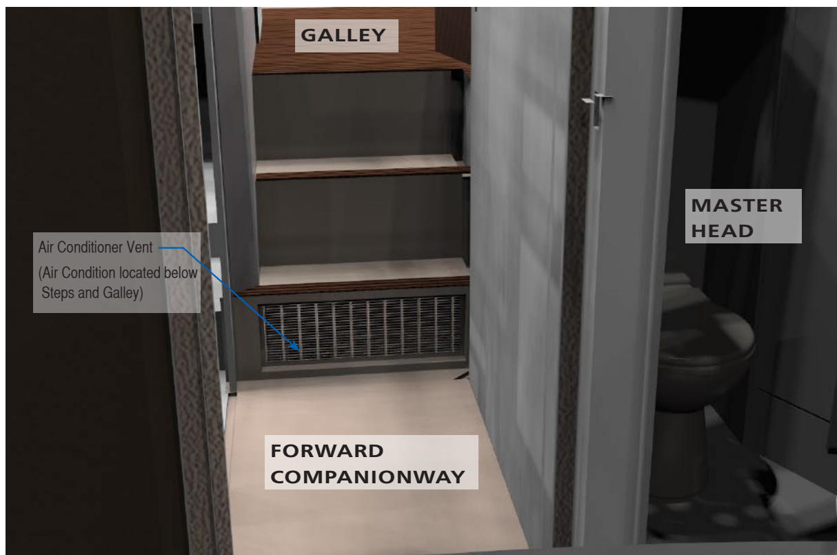
AIR CONDITIONER RETURN VENT
