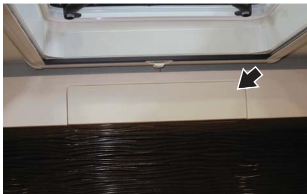
Figure 4-1 – Emergency Ladder Location
