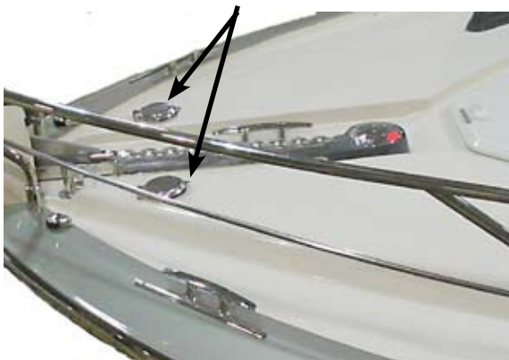
Bow Anchor Switches (lift covers to access)
