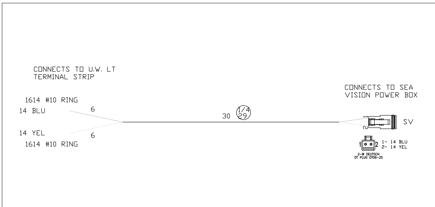
Figure 7.47 Sea Vision Power Box Exterior Harness
