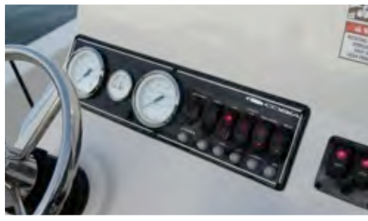
Switch Panel (above)
