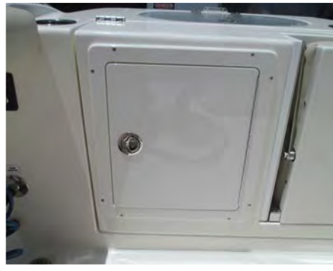
Filter Access Panel
