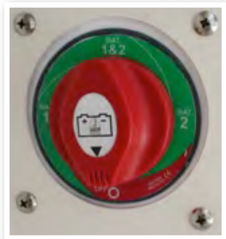
Battery Switch, Shown in the “Off” Position
