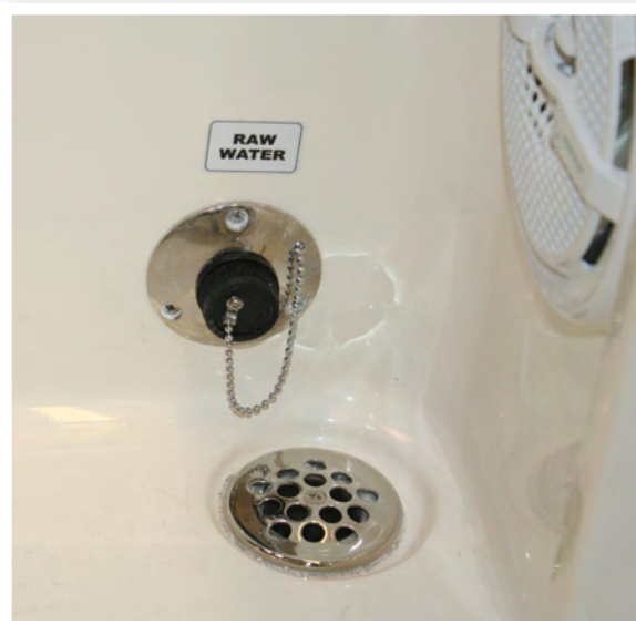
Raw Water Receptacle
