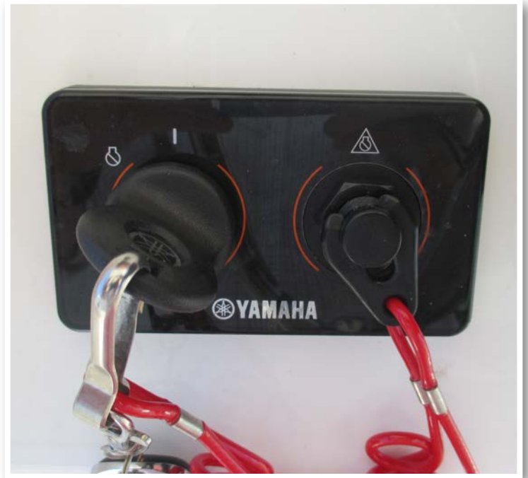
Engine stop switch (above)
