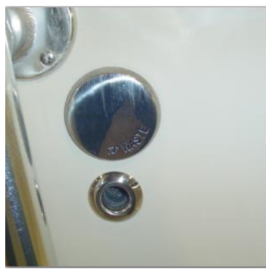
Waste Removal Fitting,
