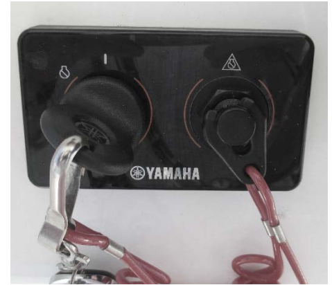
Engine Stop Switch
