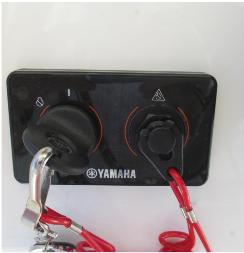
Engine stop switch (above)
