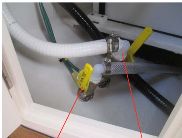
Intake Valve (open)
