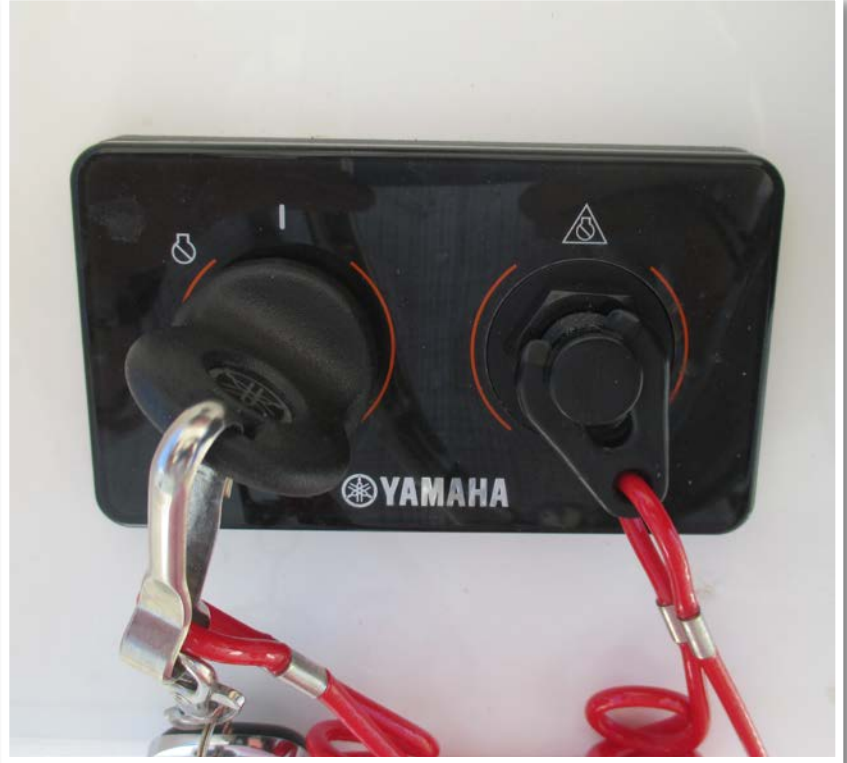
Engine stop switch (above)
