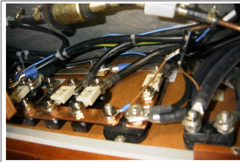
————— from left 1 = Technik Paneel 250Am 2= E-Winch BB 200Am ABB.: FUSES 3= E.-Ankorwinch 100Am 4= Distribution Navi-Place 50 Am ABB.: MAIN FUSES 1 – Anchor winch 2 – General Consumption
