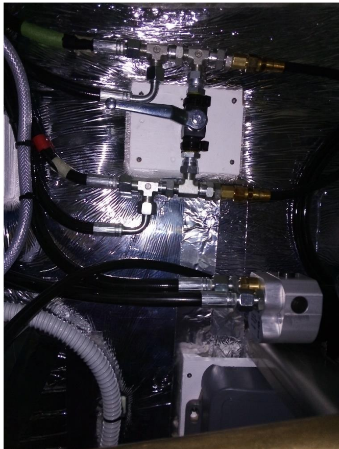
Steering by-pass for automatic pilot
