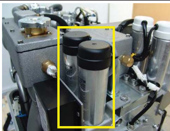
Fig. A.3.6-19: Booster capacitors 120V/60Hz
