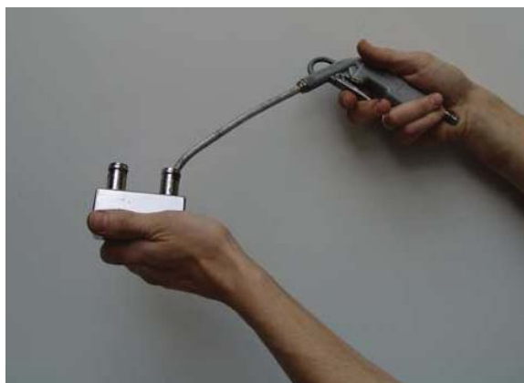
Fig. H.3-9: Cleaning with air
