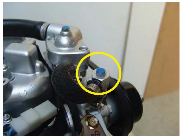
Fig. A.3.3-9: Ventilation screw cooling water pump
