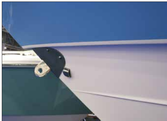
Rope Locker Drain Fitting in Hull Side
