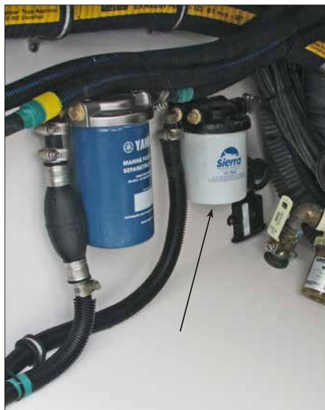
Generator Water Separator Fuel Filter
