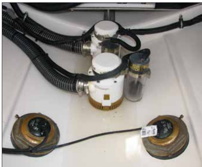
Bilge Pumps & Automatic Switches
