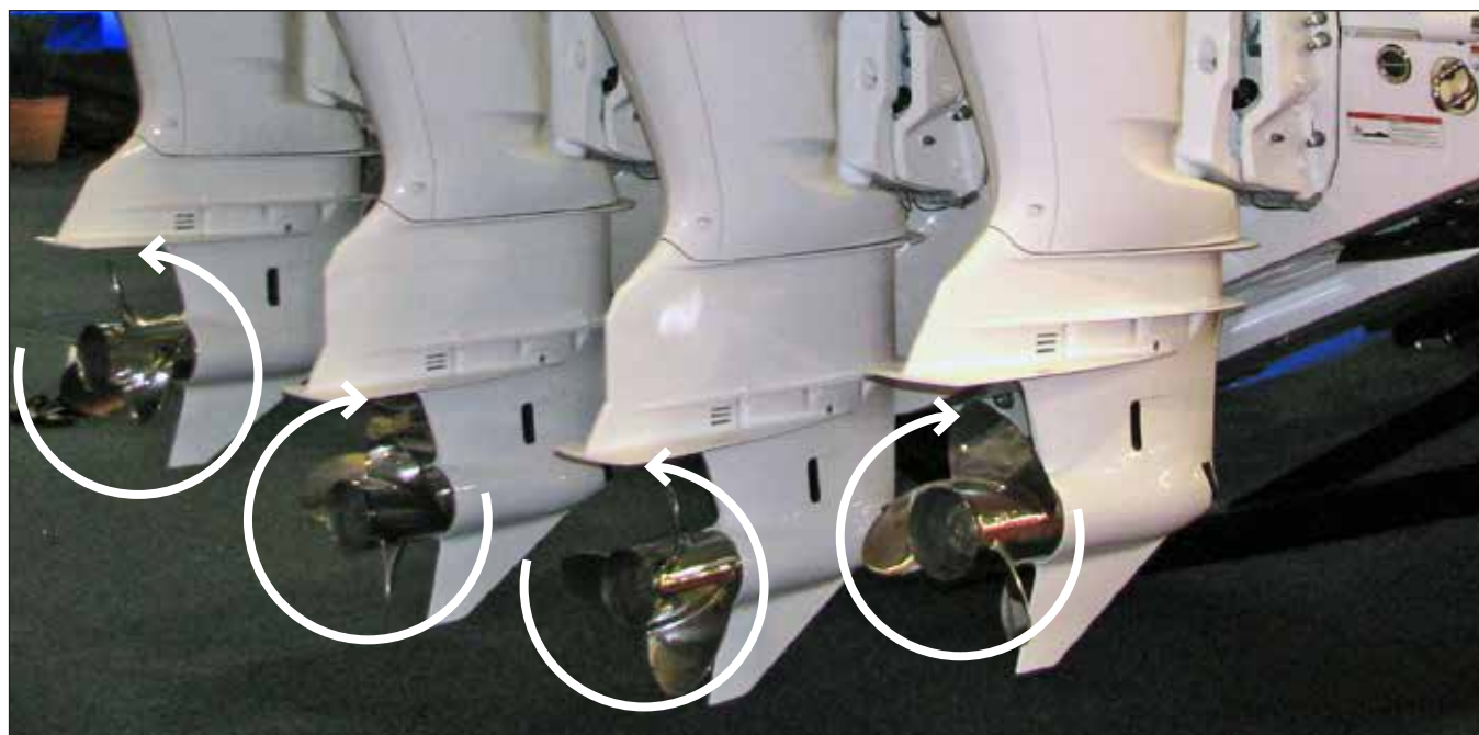
Typical Quad Engine & Propeller Rotation
