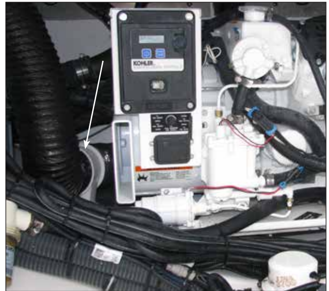
Mechanical Systems Compartment Blower
