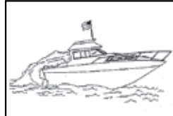
Back Drafting / Station Wagon Effect - at cruising speed with no forward ventilation
