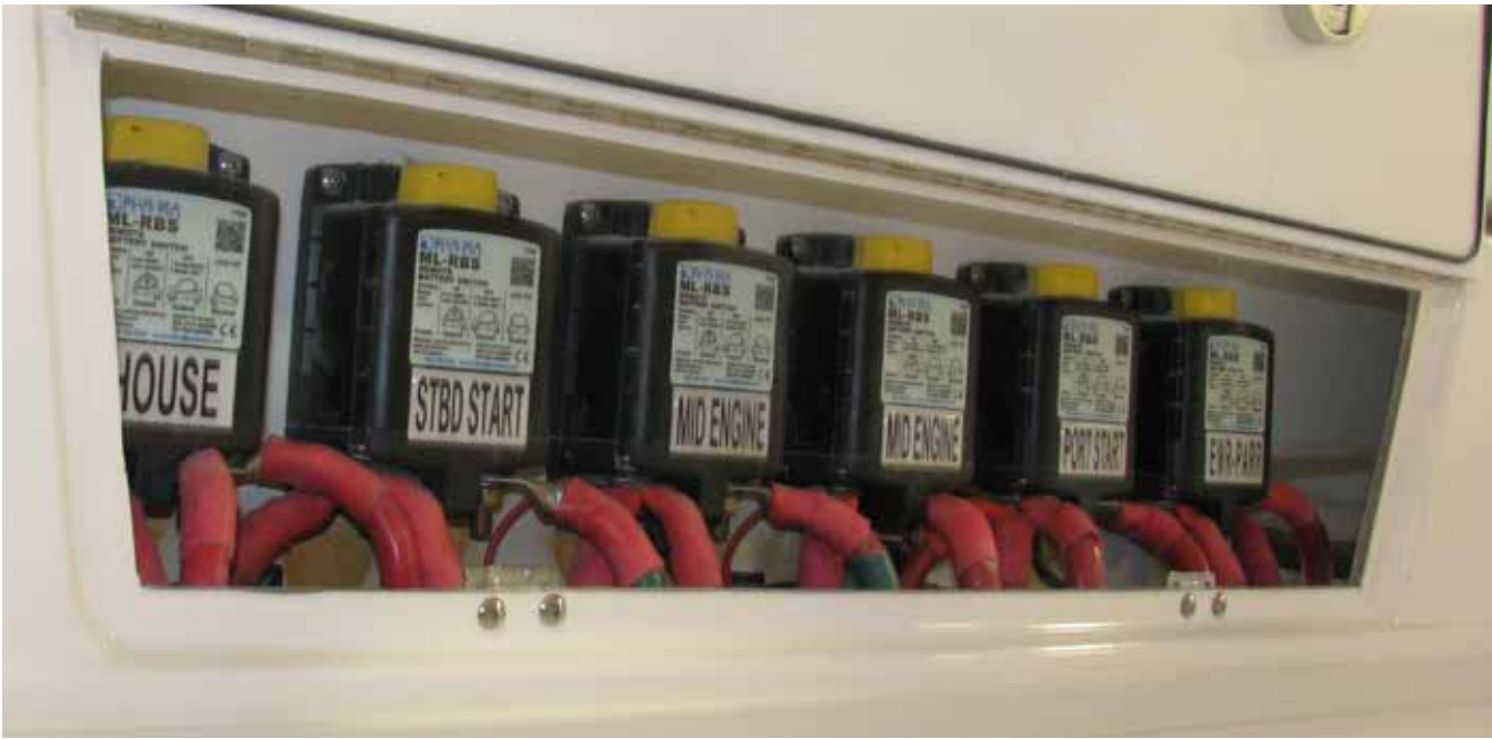
Remote Battery Switches & Emergency Parallel Switch
