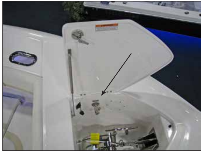
Windlass Raw Water Washdown Hose Connection
