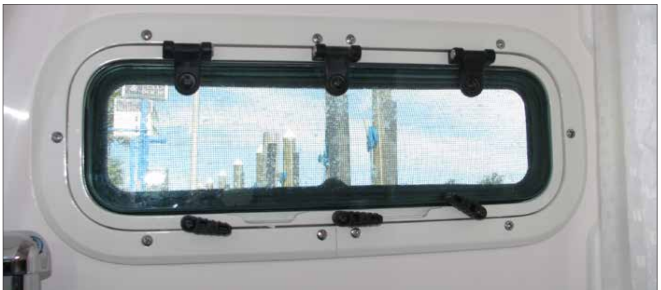
Typical Cabin Port Window
