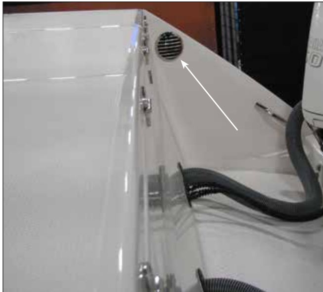
Starboard Bilge & Mechanical Systems Compartment Free Air/Forced Air Vent Aft of Cockpit
