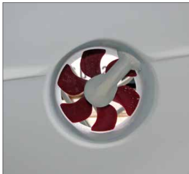
Typical Bow Thruster Drive Unit, propeller & tunnel
