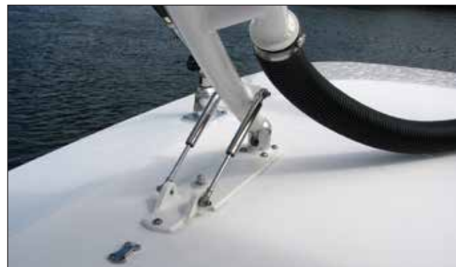
Gas Charged Assist Springs
