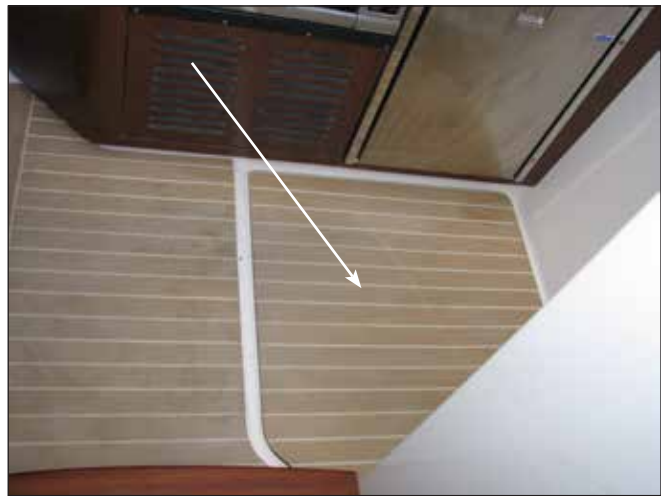
Removable Cabin Floor Panel Remove To Access Bilge Pump & Drain Sump Pump
