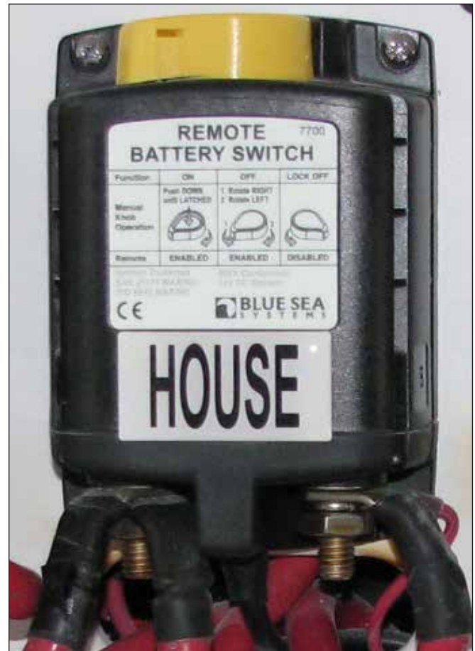
Typical Remote Battery Switch
