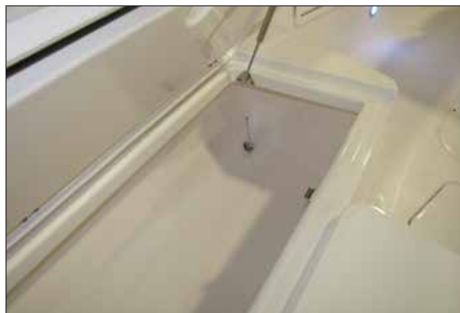
Bow Storage Compartment Drain & Drain Plug
