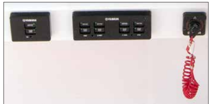
Yamaha Quad Engine Stop Switch & Lanyard Ignition START/STOP Switches
