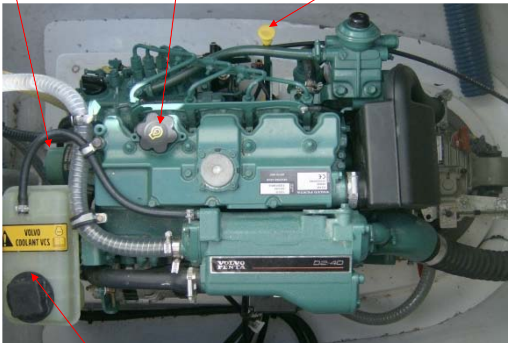
Coolant tank and
