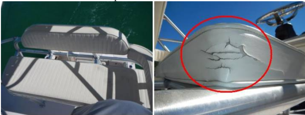
Large bench seat. Corner of the bench on the starboard side has cracked vinyl. Good Condition.
