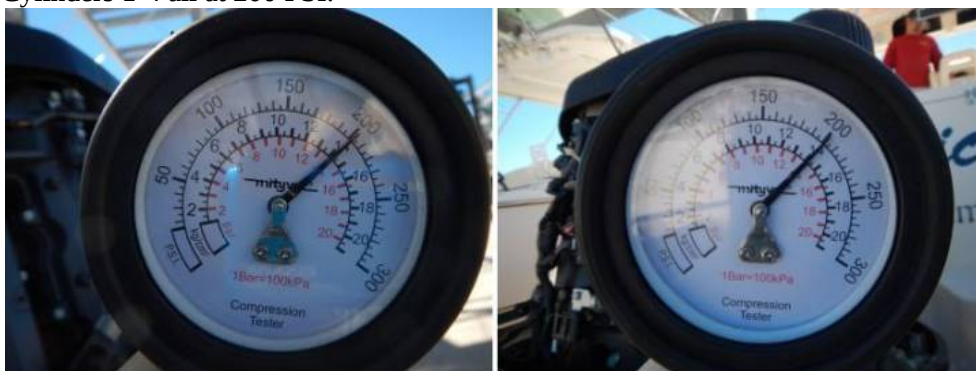
Cylinders 5-6 at 200 PSI.
