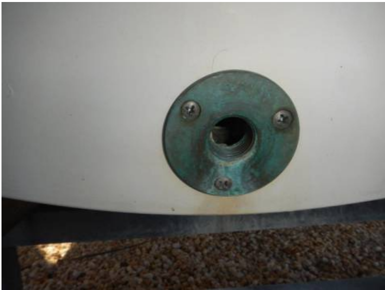
Transom mounted bronze drain plug fitting.
