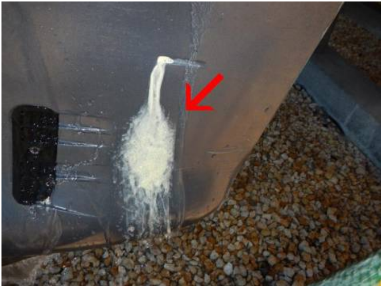
Starboard engine running while on fresh water flush out. Milky lower unit oil is seeping out of the unit.
