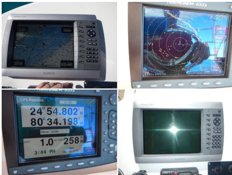
Northstar 6000 on the main helm and Garmin GPS Map 4210 on the flybridge. Units powered up and operated during the sea trial.
