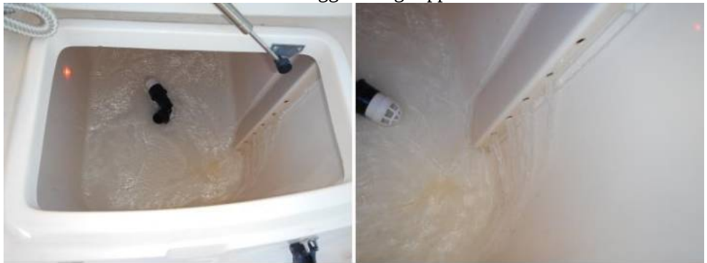
Live well pump powered up and functioned. Capacity unknown.
