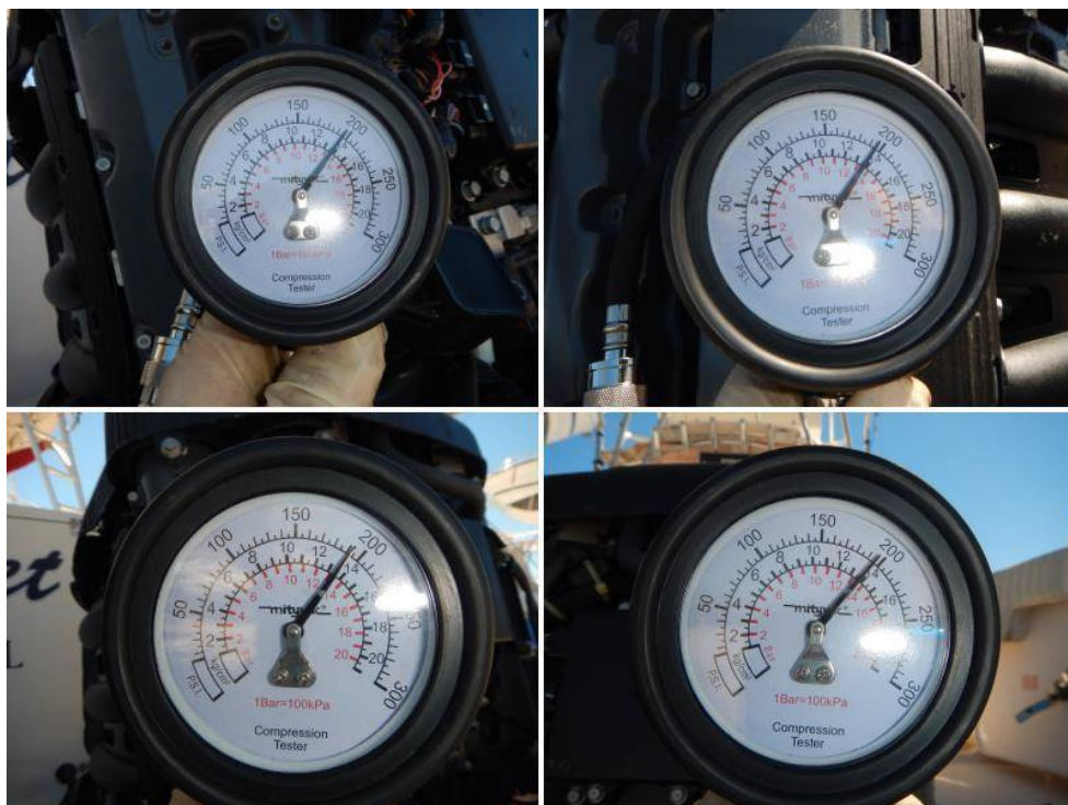
Cylinders 1-2-4 at 200 PSI and cylinder 3 at 199 PSI.
