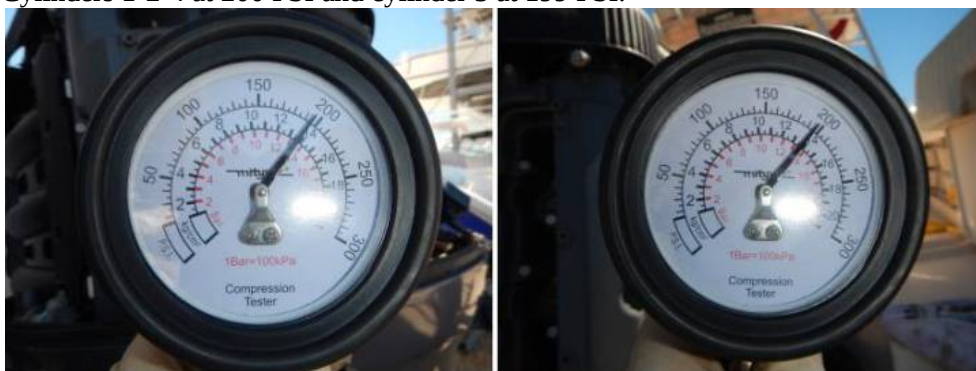
Cylinders at 200 PSI.
