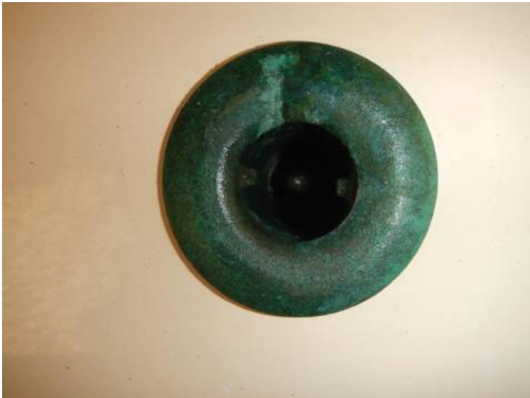
Mushroom type bronze fittings for all below water line sea cock locations. Well secured to hull bottom.
