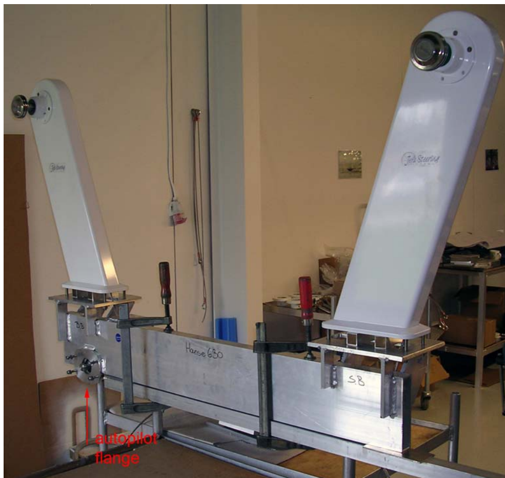
Setup of the traverse system. At the left the autopilot flange is visible.
