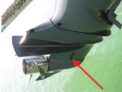
Sea water intake Located directly on the saildrive
