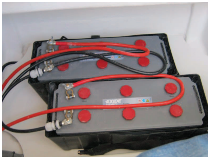
Engine battery : 140A - Single engine Engine battery: 2 x 140A - Twin engine
