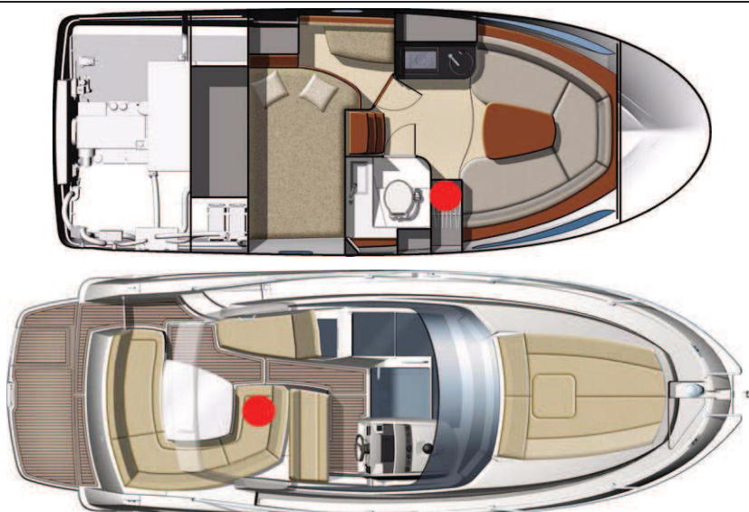
Recommended positioning of portable extinguishers (not supplied): -Saloon cupboard -Cockpit locker
