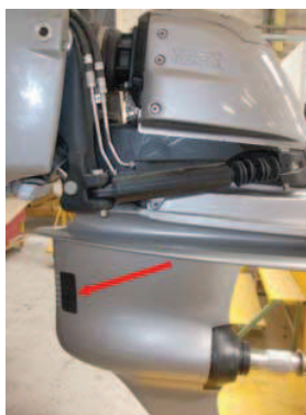
Sea water inlet valve for engine Located directly on the housing
