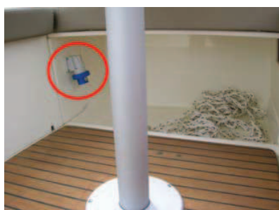
Shore power socket 220V - 16A
