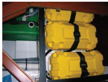
Propeller battery: 2 x 50A
