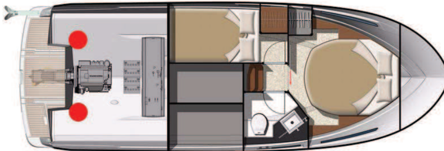
Position of fixed extinguishers
