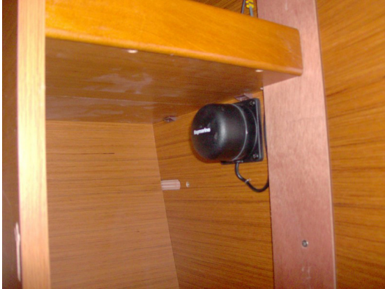
Gyrocompass - Hanging locker - Aft cabin
