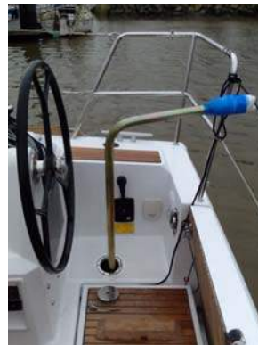
Emergency tiller - in position
