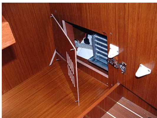
Access hatch - Refrigeration unit
