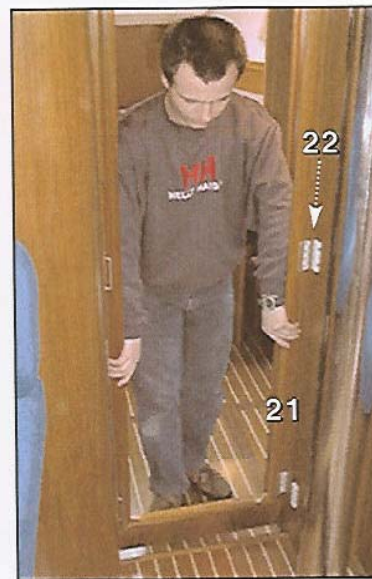
21- Take the door 4 off its hinges to position the door frame.
