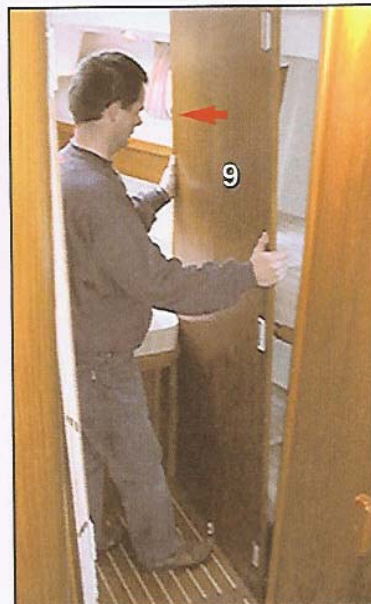
9- Dislodge the lateral bulkhead. This bulkhead is hinge mounted and can be folded up. Put it aside.
