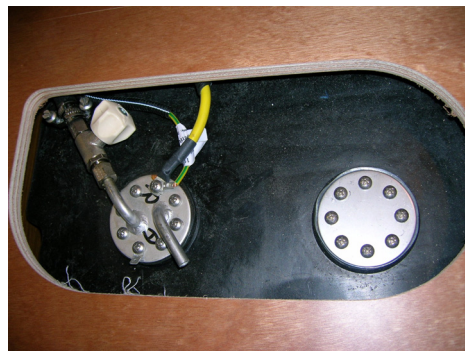
Fuel oil valve for engine
