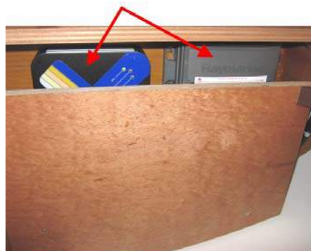
Elements - AIS Location: Under map table
