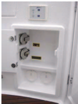
AC sockets (Shore / Air conditioning) Ref 1
