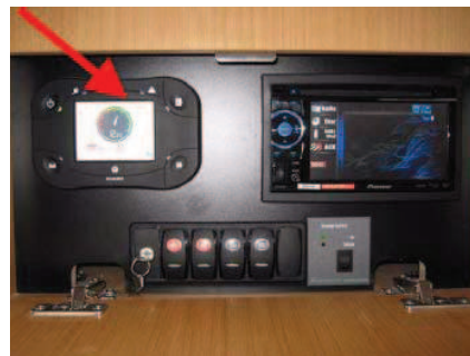
Control - AC Source selector (See Lighting chapter - Touch screen) Ref 2
