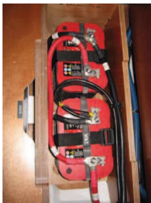
Battery - Bow thruster: 2 x 50A
