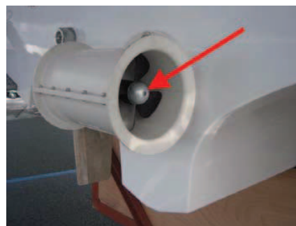
Anode - Stern thruster
