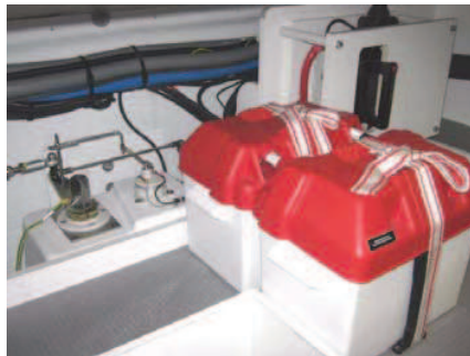
Battery - Bow thruster: 2 x 50A
