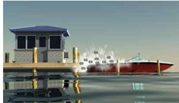
Blockage of boat exhaust by obstruction.
