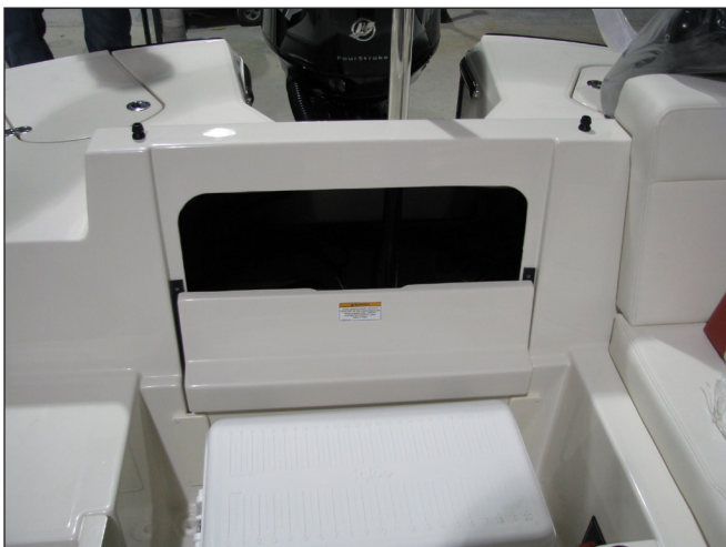
197BF/217BF Cooler Storage Compartment & Bilge Close Out Panel
