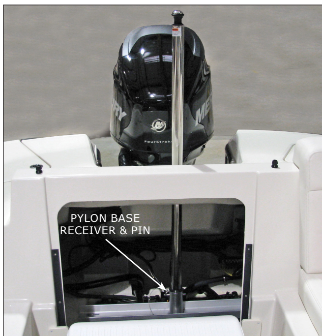
Outboard Ski Tow Pylon Installation
