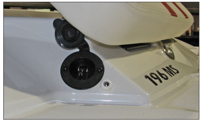
196MFS Battery Charger Shore Cable Inlet Plug
