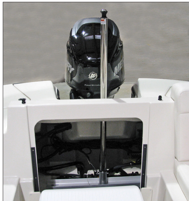
197BF/217BF Bilge Access - Close Out Panel Removed
