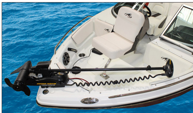
Typical Trolling Motor Mounted to Deck
