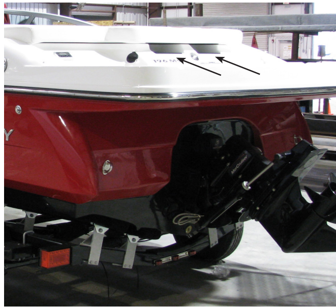
196MFS Engine Compartment Vents
