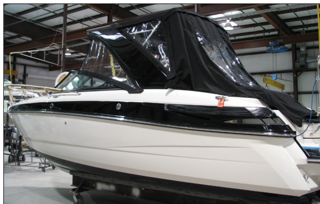
264FSC Arch Canvas & Clear Connector Installed Note that front clear connector attaches directly to arch.
