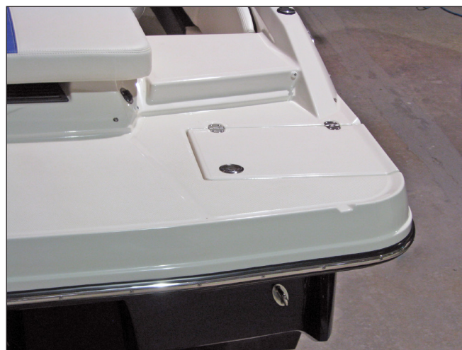
Typical Inboard Stern Ladder Compartment on Platform
