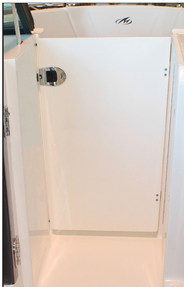
264FS/264FSX Helm Storage Compartment Door & Walk-Thru Door Latched Open - Walk-Thru Closed Off
