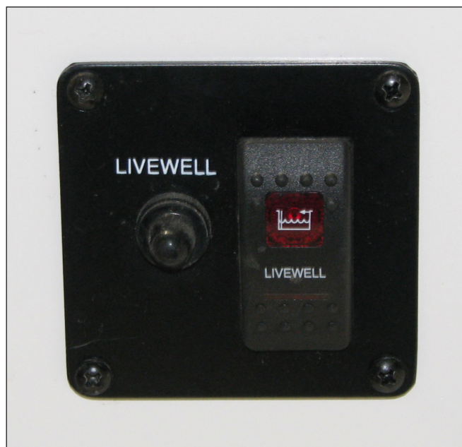
Livewell Switch & Circuit Breaker
