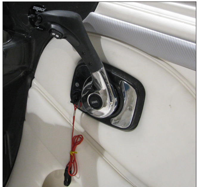
Typical Volvo Inboard Side Mount Cable Control & Stop Switch
