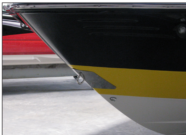
Typical Rope Locker Drain
