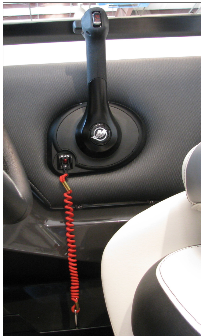
Mercury Outboard or Mercruiser Inboard Control, Emergency Stop Switch & Lanyard
