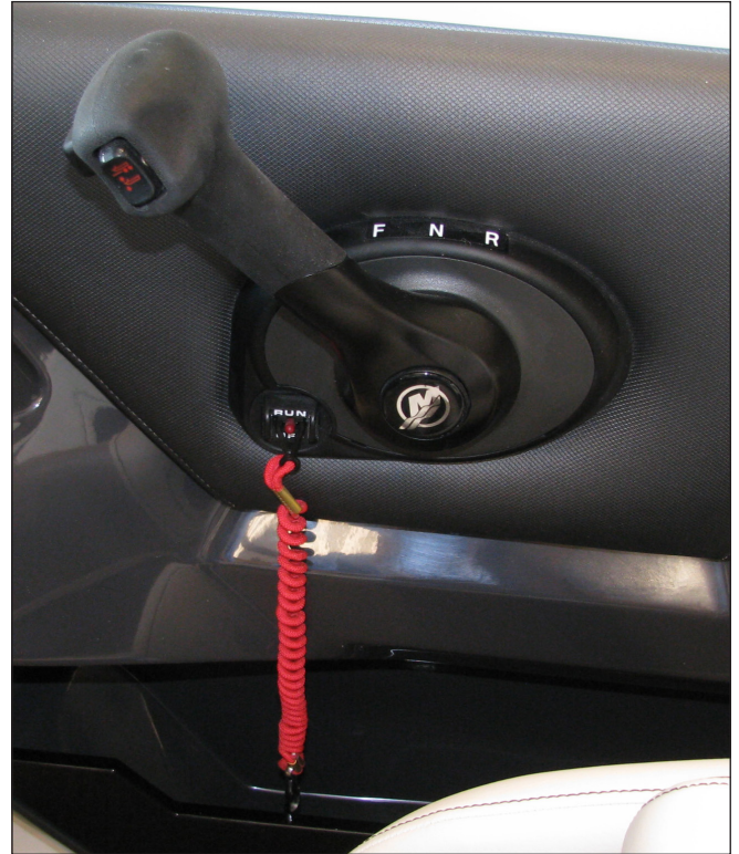
Typical Mercury Outboard or Mercruiser Inboard Side Mount Cable Control & Stop Switch
