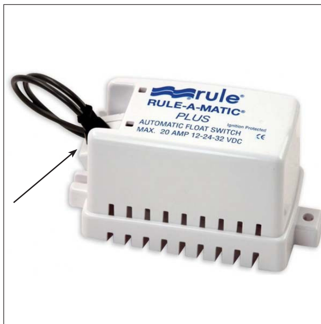
264FSC High Water Alarm Float Switch Test Button Push Button Down & Hold Until Pump & Alarm Activate
