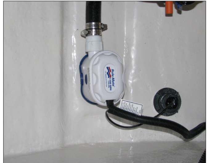
Typical Automatic Bilge Pump
