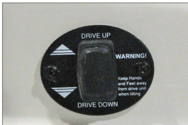
Typical Outdrive Tilt Switch Near Transom Door
