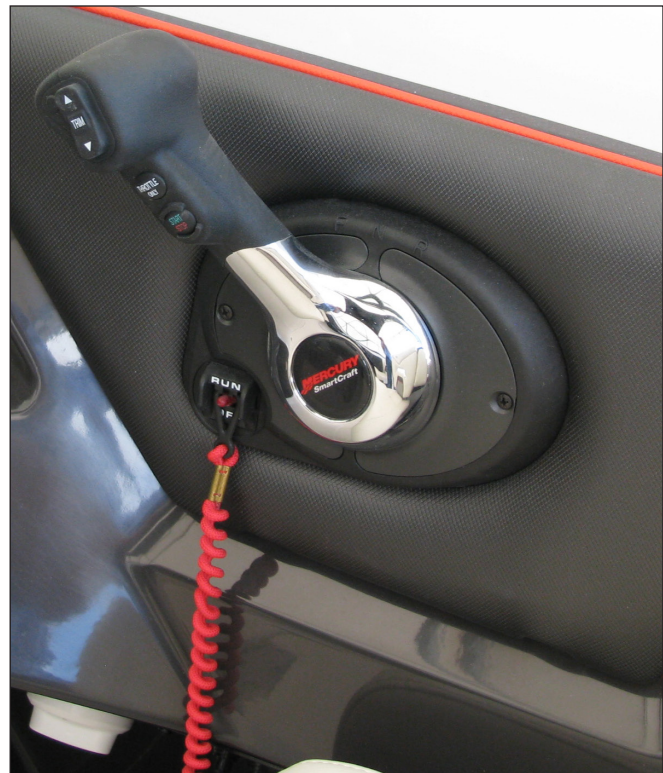
Typical Mercury Outboard or Mercruiser Inboard Side Mount Electronic Control & Stop Switch
