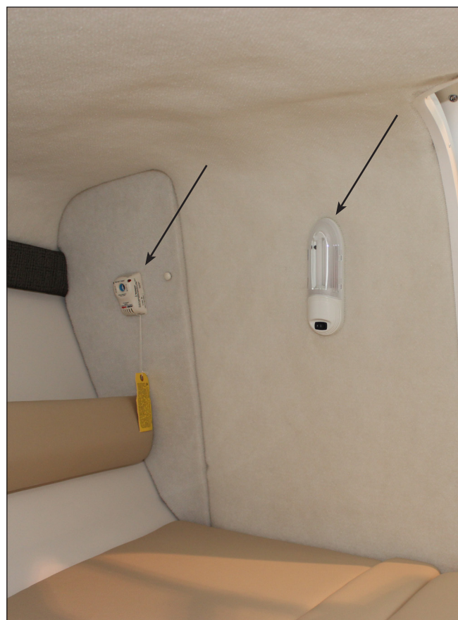
Cabin Light & Carbon Monoxide Detector
