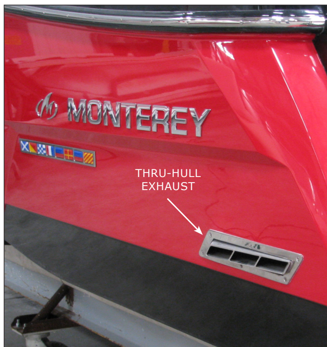
Typical Thru-Hull Exhaust Port
