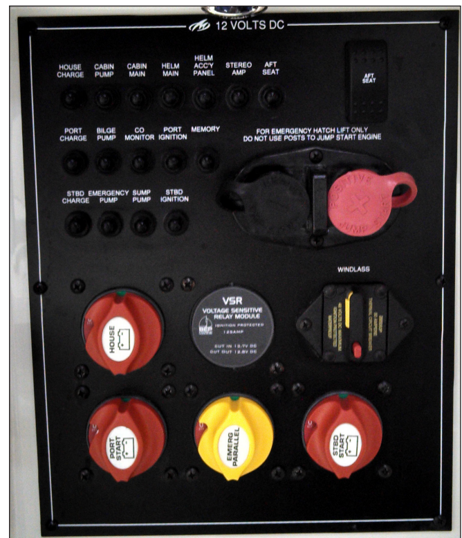
328SS Battery Switch Panel, Circuit Protection & Switches
