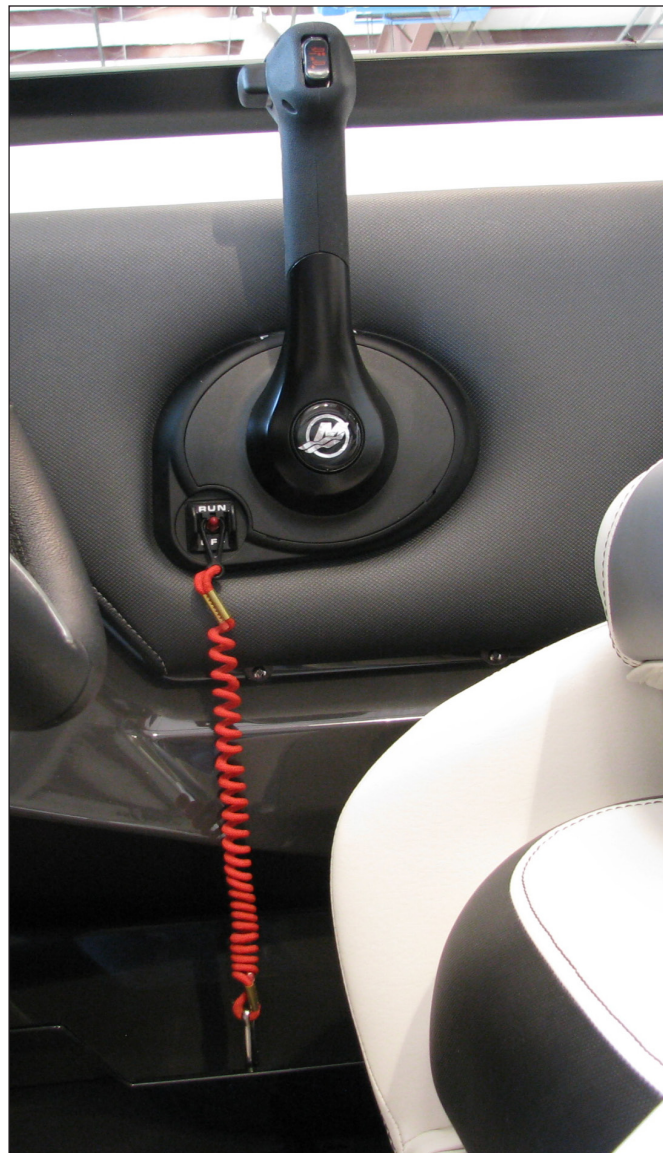
Mercruiser Control Emergency Stop Switch & Lanyard
