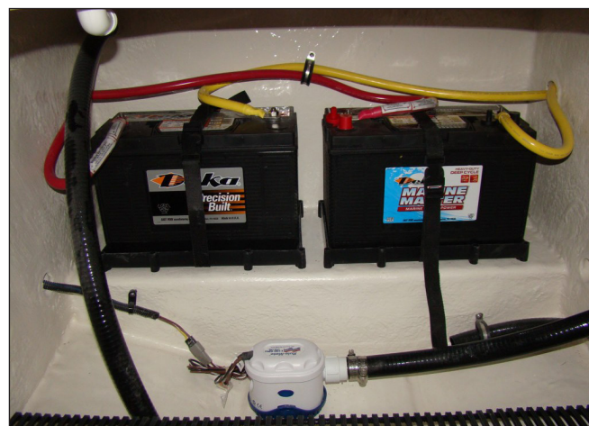
288SS Forward Automatic Bilge Pump
