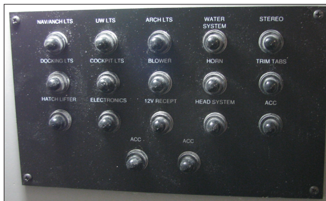
268SS Helm Accessory Circuit Breaker Panel
