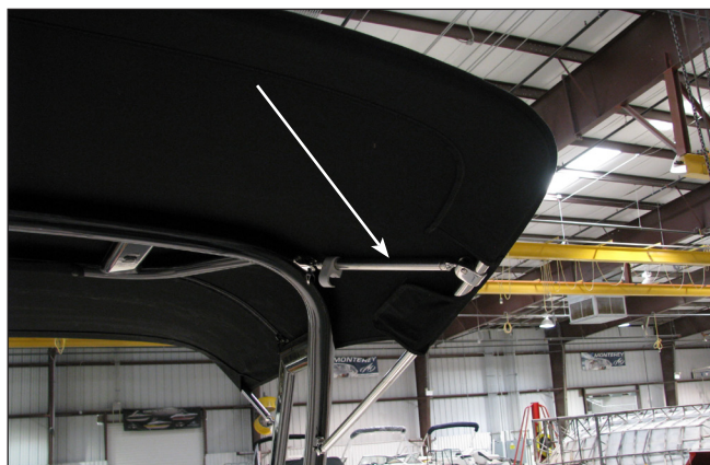
Front Top Open & Supported With Stanchion
