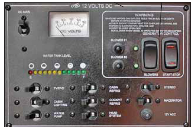
DC Electrical System W/ Optional Generator Control Panel
