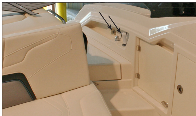
328SS Cockpit Shower Head & Shower Water Connection
