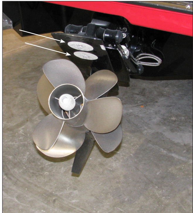
Typical Mercruiser Outdrive Anodes
