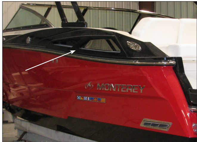
Typical Engine Compartment Vents
