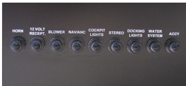
Helm Accessory Circuit Breaker Panel 214SS/218SS & 234SS/238SS
