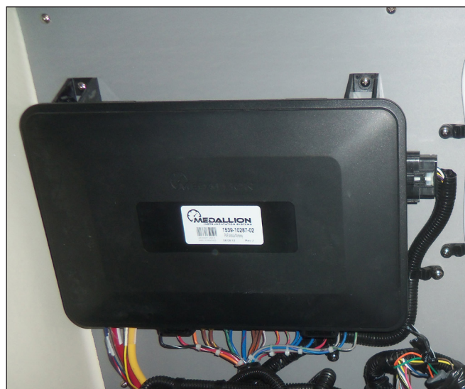
Power Management Module with Cover On
