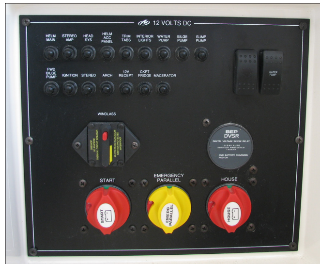
288SS Battery Switch Panel, Circuit Protection & Switches
