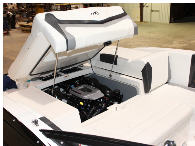
Engine Access 214SS/218SS & 234SS/238SS
