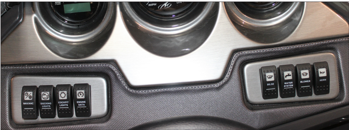
Helm Switch Panels 214SS/218SS & 234SS/238SS
