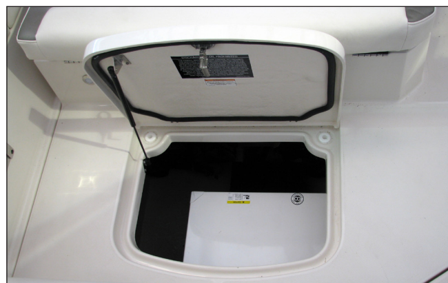
315SY Engine Compartment Day Hatch
