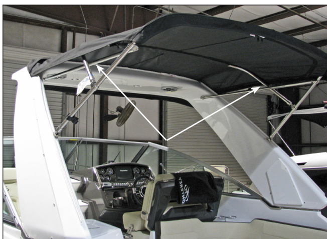
275/295SY Rear Top Extended & Rear Adjustable Stanchions
