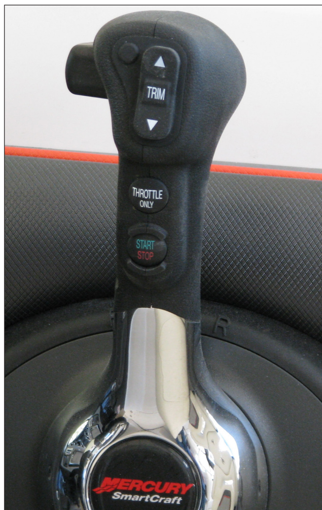
Mercuriser Single Engine Tilt/Trim Switch
