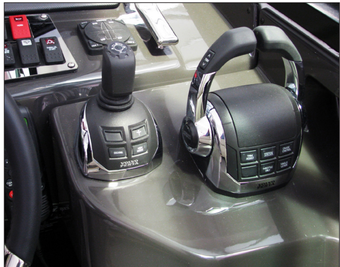
Typical Volvo Joystick & Binnacle Controls
