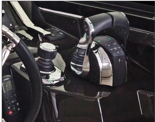
Typical Mercruiser Joystick & Binnacle Controls
