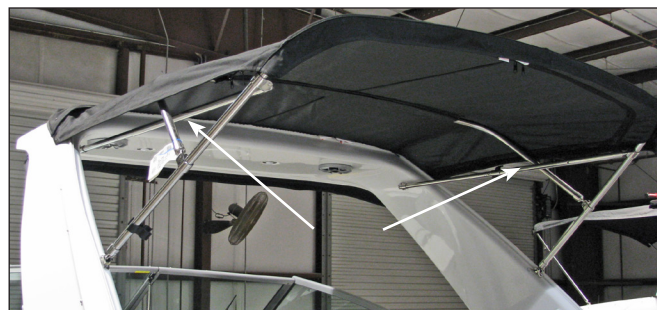
Typical Rear Top Section Extended & Adjustable Stanchions
