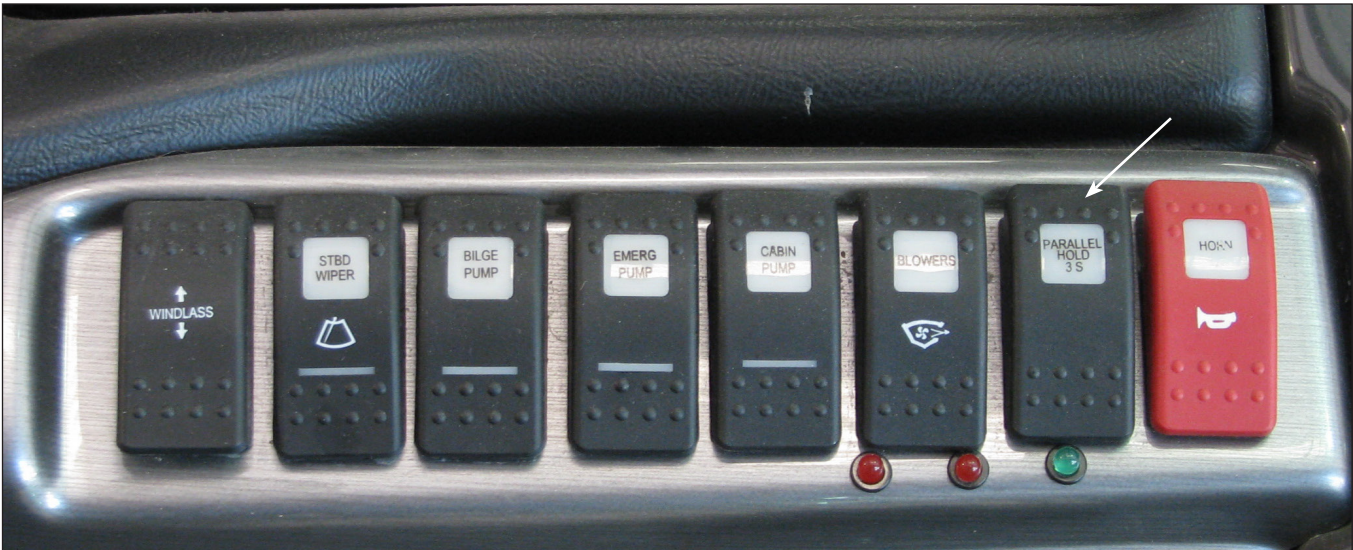
Helm Switch Panel & Parallel Start Switch
