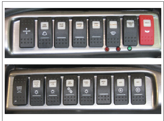
Typical 315SY Helm Switch Panel
