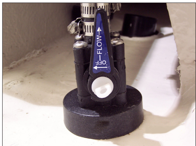
Air Conditioner Seacock (Thru-Hull Valve)
