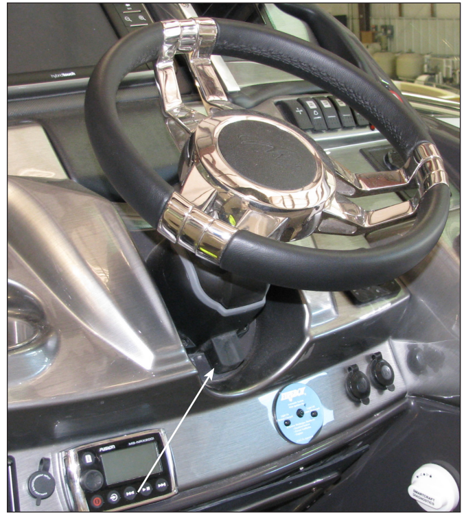
Tilt Steering Wheel & Tilt Release Lever
