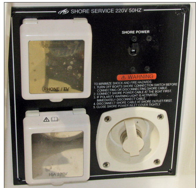
275/295SY 220 Volt AC Inlet Panel With ELCI
