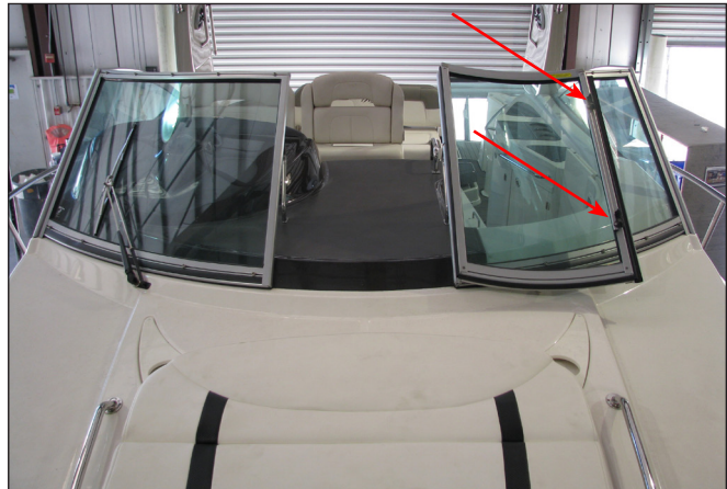
315SY Windshield Walk-Thru Panel & Cam Locks
