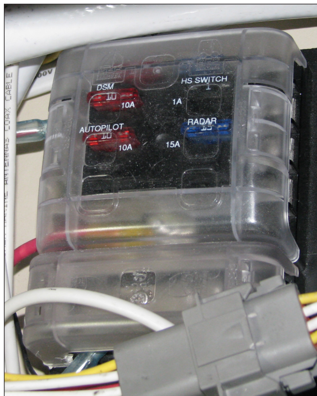
Typical Fuse Panel for Optional Electronics
