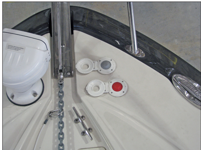
Anchor Line Cleat & UP/Down Deck Foot Switches
