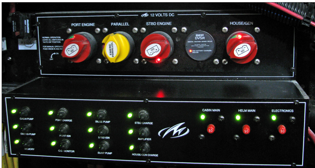
315SY Battery Switches & Battery Switch Circuit Breaker Panel
