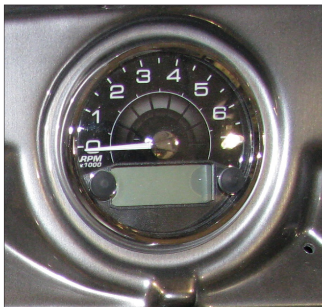
Typical Digital Analog Tachometer & LCD Screen
