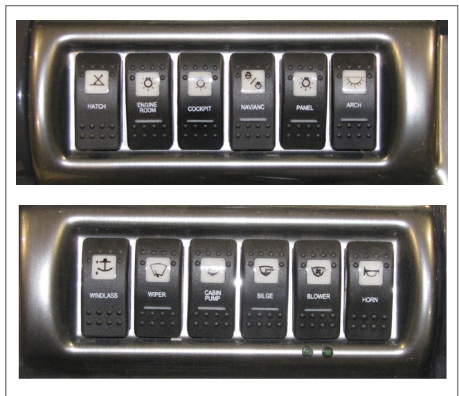
Typical 275SY Helm Switch Panel
