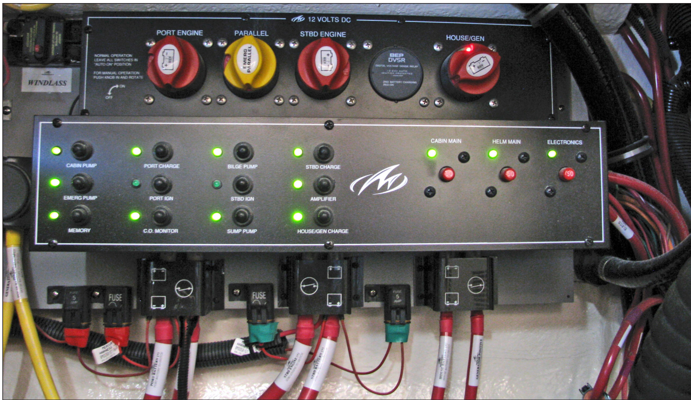
Battery Switch Panel, Battery & Parallel Switches, Main Circuit Breakers & Continuous Duty Circuit Breakers
