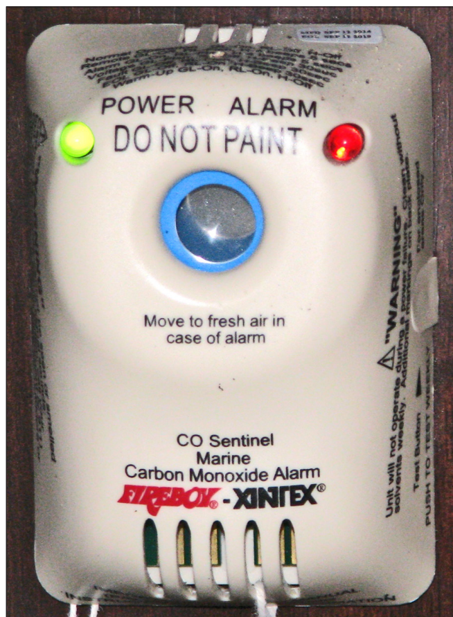
Cabin Carbon Monoxide Detector
