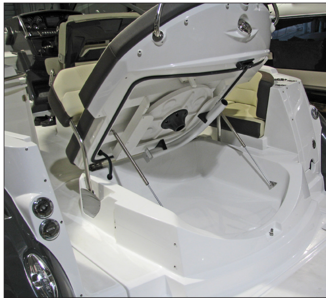
Typical Transom Storage Compartment Below Sun Lounge
