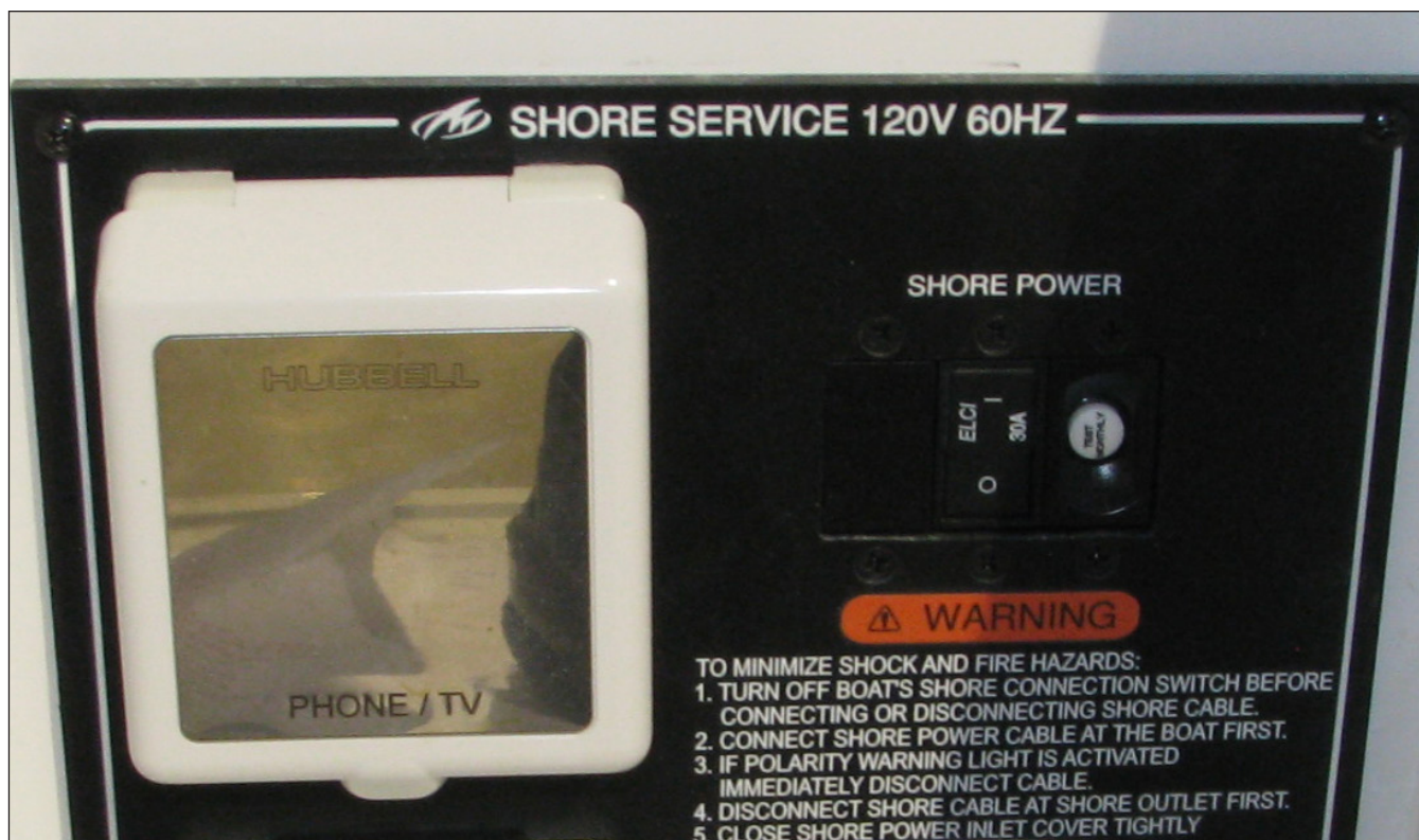
275/295 Inlet Panel ELCI Circuit Interrupter/Circuit Breaker
