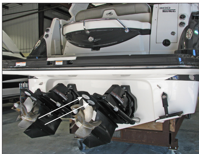
Typical Mercruiser Outdrive Anodes
