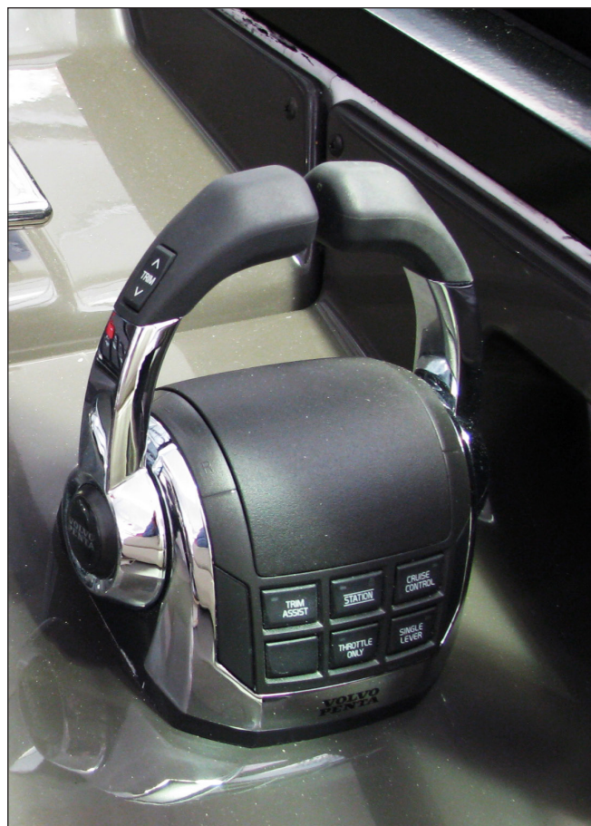
Typical Volvo Dual Engine Binnacle Control
