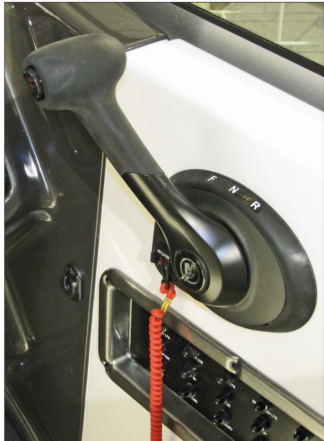
Mercruiser Side Mount Cable Control & Stop Switch
