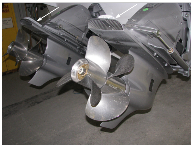
Typical Volvo Outdrive Anodes
