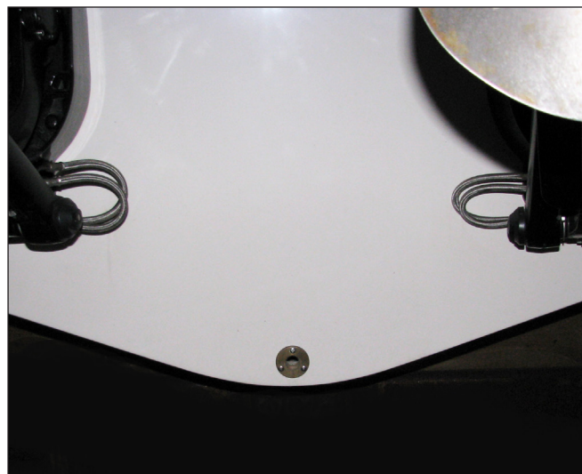
Typical Bilge Drain Plug In Transom
