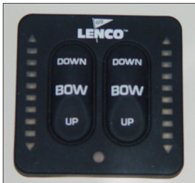
Standard Trim Tab Control Switch Panel
