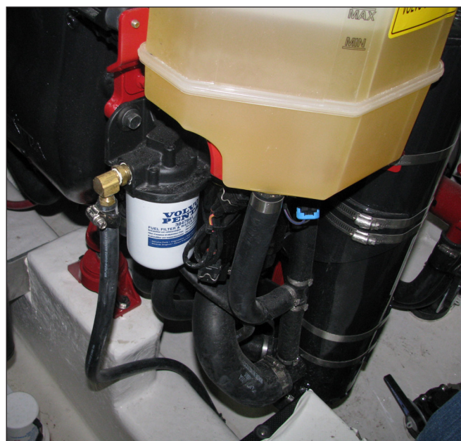
Typical Spin On Engine Fuel Filter
