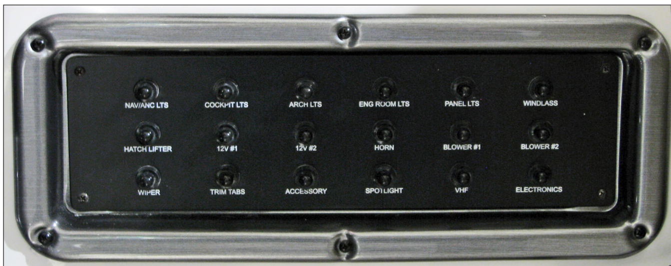
275/295SYSY Helm Circuit Breaker Panel
