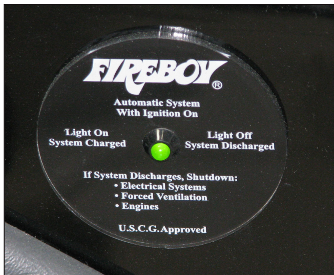
Fire Extinguisher Panel In Helm
