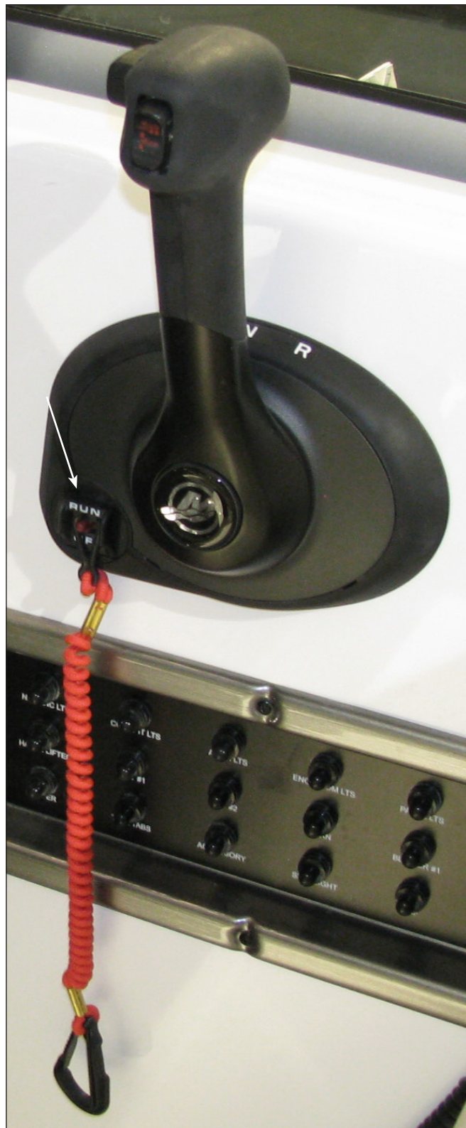
Mercruiser Control Emergency Stop Switch & Lanyard
