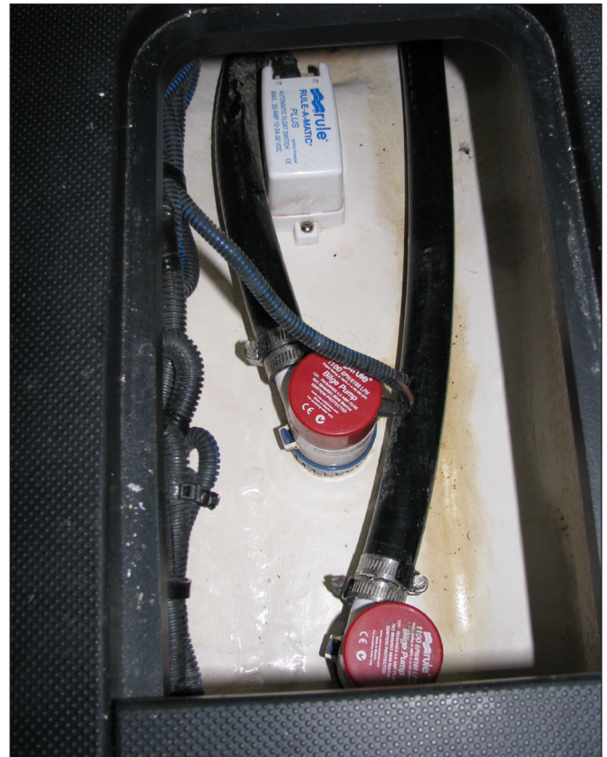
315SY Aft Bilge Pump, Emergency Bilge Pump & Aft Pump Automatic Switch In The Stern Bilge Between The Engines
