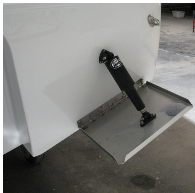
Typical Trim Tab Plane, Actuator & Sacrificial Anode
