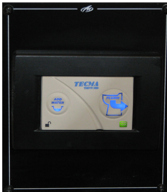
Head Compartment Toilet Control Panel
