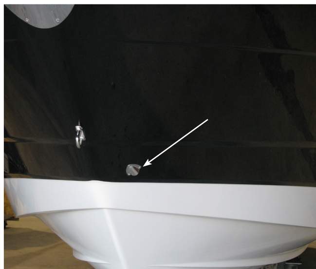
275/295SY Rope Locker Drain
