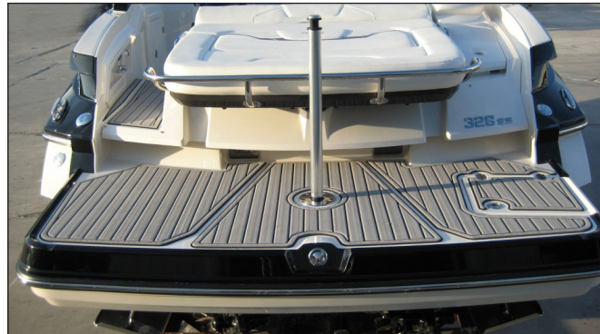
Typical Platform Ski Tow Pylon
