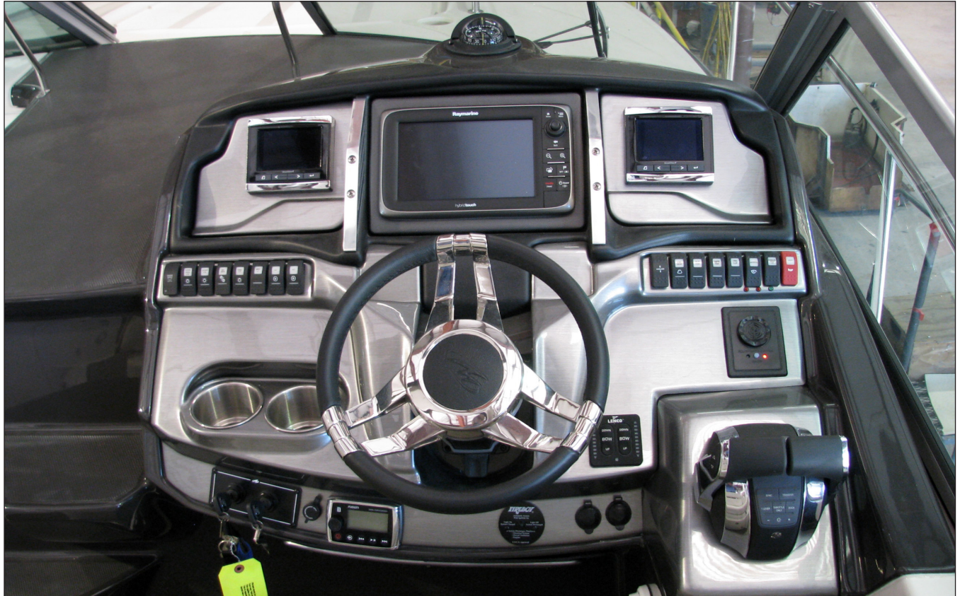
315SY SY Helm & Instrument Panel With LCD Multifunction Displays
