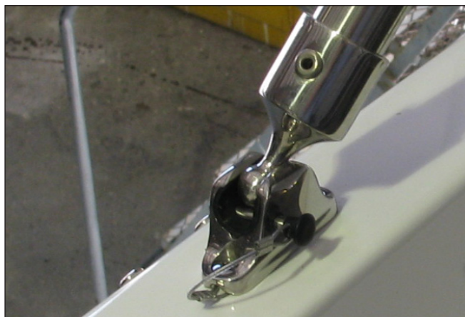
Typical Stanchion Ball End, Deck Hinge & Quick Release Pin
