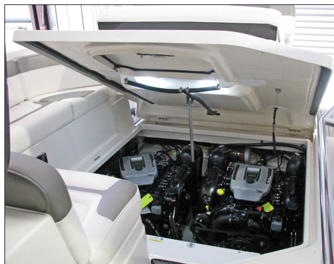
315SY Engine Compartment Hatches & Hatch Lifter
