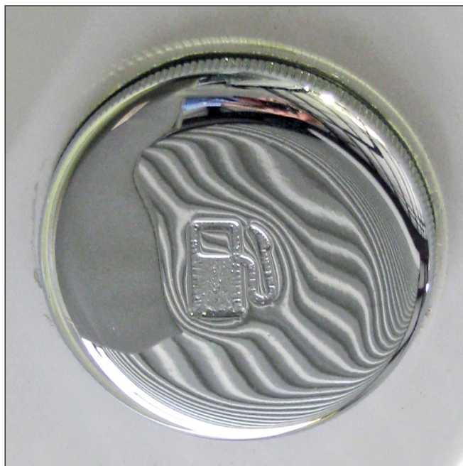
Typical Keyless Fuel Fill
