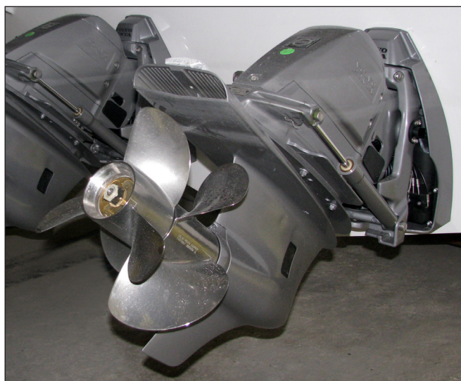
Typical Volvo DP Propellers
