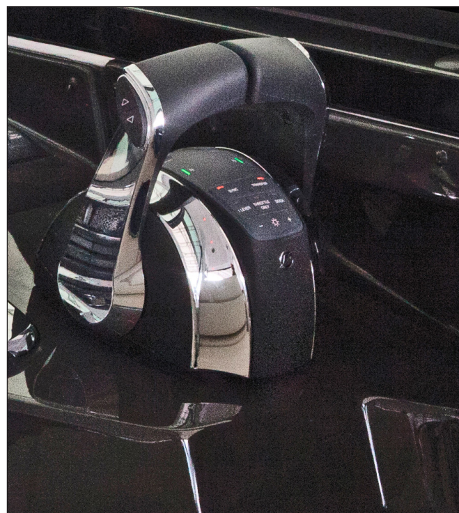
Typical Mercruiser Dual Engine Binnacle Control
