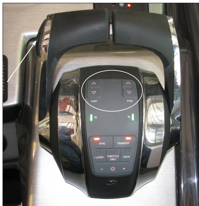
Mercuriser Twin Engine Tilt/Trim Switches
