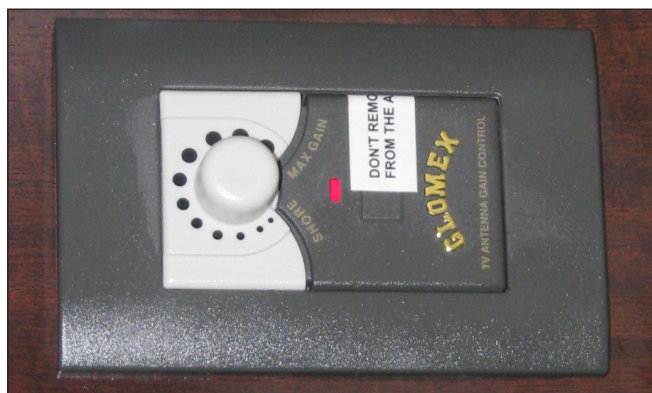
TV Antenna Gain Control
