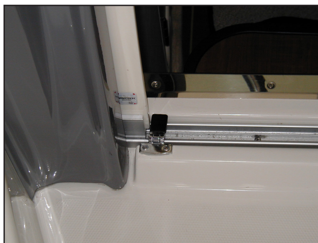
Cabin Door Latched in the Open Position
