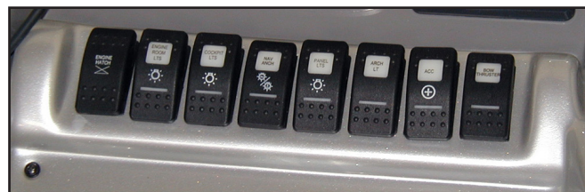
Helm Switch Panel - Port Side
