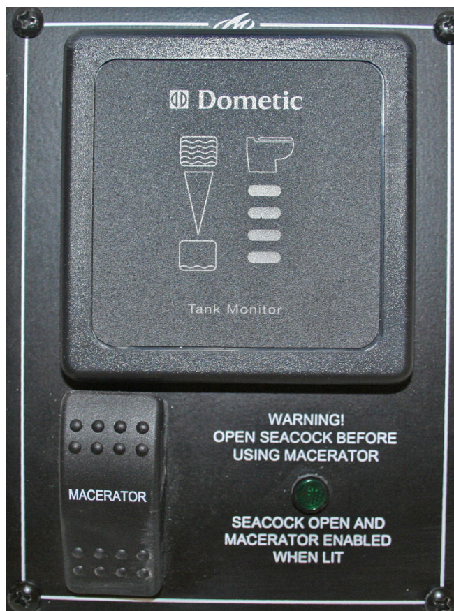
Holding Tank Monitor Panel
