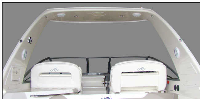
Rear View of Fiberglass Arch
