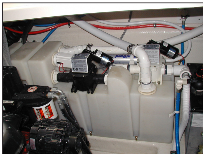
Holding Tank, Vacuum Pump and Overboard Macerator Pump
