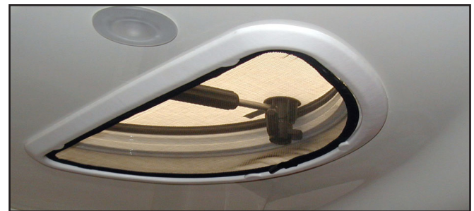
Galley Hatch Fully Closed Screen Installed
