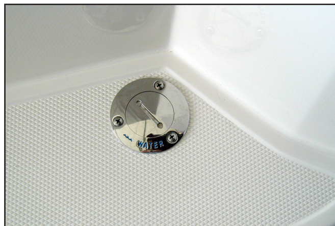
Fresh Water Fill
