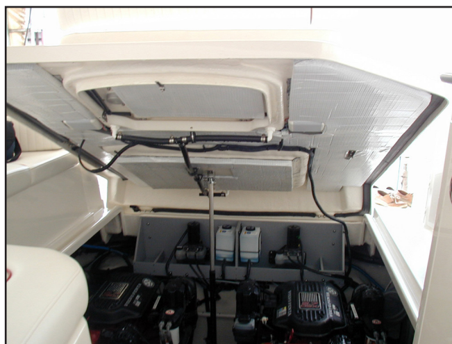
Engine Compartment Hatch, Day Hatch and Cockpit Drain System
