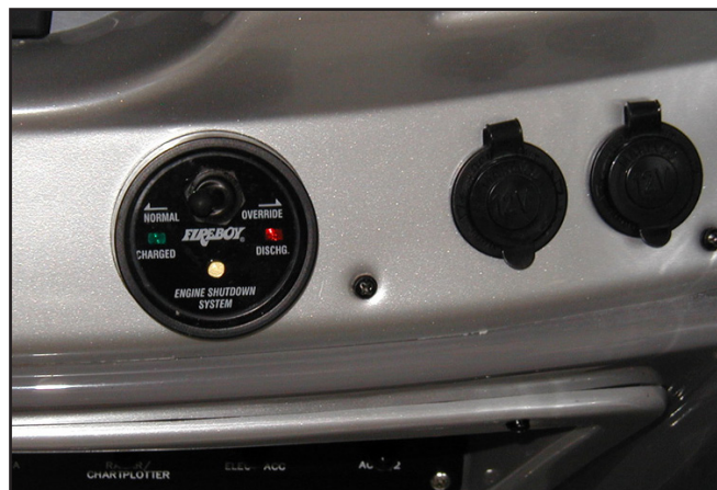
Override Switch and Fire Extinguisher Indicator Lights
