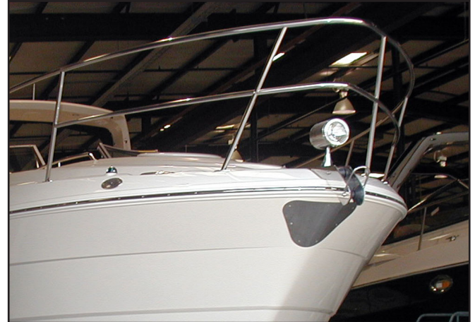
Roller Assembly, Spot Light and Bow Rail
