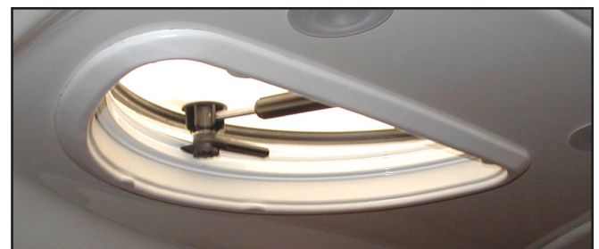
Galley Deck Hatch Secured in Vent Position
