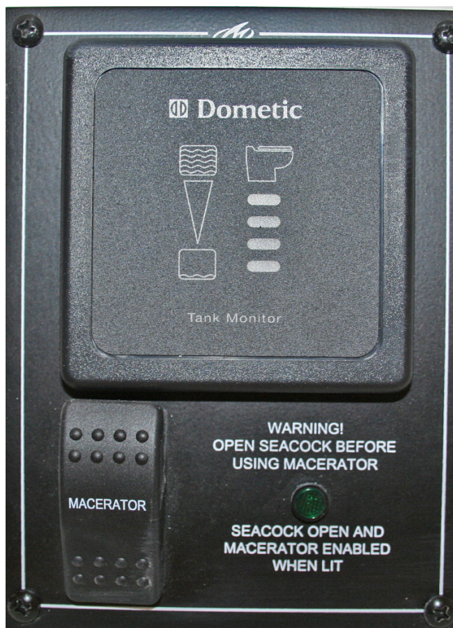
Holding Tank Monitor Panel
